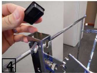
Place the black plastic cap on the "Upright Bracket".
