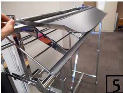
Lay the black styrene sheet in the shoe shelf to prevent shoes from slipping through.
