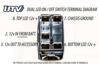
THIS WILL TURN THE TOP LED ON WHEN THE SWITCH IS ACTIVATED AND TUEN THE LED OFF WHEN THE SWITCH IS OFF. WE NORMALLY PULL 12v + AT TERMINAL 6 FROM A KEYED IGNITION SOURCE TO ILLUMINATE THE LOWER LED. THIS WAY YOU CAN TURN YOUR ACCESSORY ON WITHOUT HAVING TO TURN THE KEY ON.
