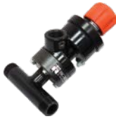
PN: 888-2149-508PB APV BIG-BORE™ METERING VALVE, 1½", W/TUNGSTEN CARBIDE SLEEVE
