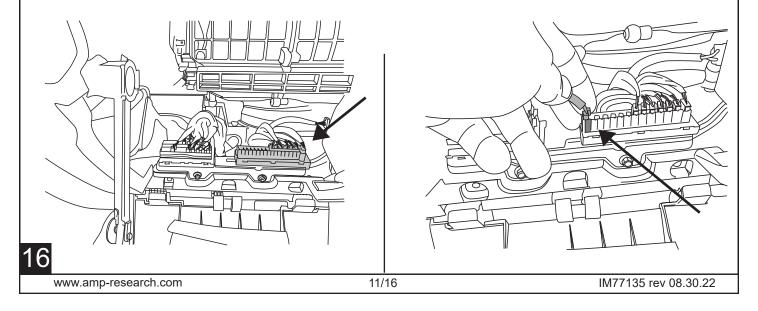
Pull back carpet on passenger side on the top side of middle console and then use provided Tube (9) to route OBD II Extension (8) behind middle console. Tape open end of extension to the tube and push the tube through middle console.
