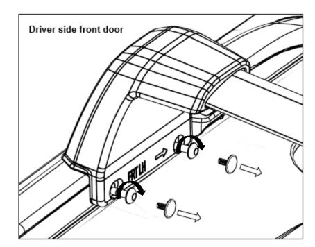
Above the driver's and passenger's side front door, locate the set of attachment locations on roof rack. Remove tree clips to expose mounting threads and install the "FRT LH" and "FRT RH" casting to this location by fastening two T-30 torx bolts (4) on each side.
