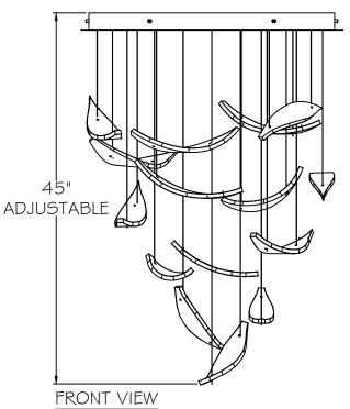
ONCE ALL GLASSES ARE INSTALLED AND FINAL GLASS POSITION IS ACHIEVED, ENSURE TO CUT EXCESS CABLES UP TO HARDWARE OF LOWEST GLASSES. REFERENCE INSTALLATION INSTRUCTIONS.
