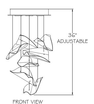
ONCE ALL GLASSES ARE INSTALLED AND FINAL GLASS POSITION IS ACHIEVED, ENSURE TO CUT EXCESS CABLES UP TO HARDWARE OF LOWEST GLASSES. REFERENCE INSTALLATION INSTRUCTIONS.
