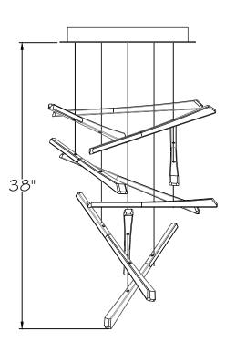
ONCE ALL GLASSES ARE INSTALLED AND FINAL GLASS POSITION IS ACHIEVED, ENSURE TO CUT EXCESS CABLES UP TO HARDWARE OF LOWEST GLASSES. REFERENCE INSTALLATION INSTRUCTIONS.
