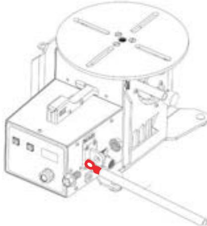
**Warning:** Failure to attach a weld ground cable directly to the unit while welding on the turntable, may cause damage to the unit. Reversely, leaving the ground cable attached to the unit while welding a part not on the turntable, may cause damage to the unit.
