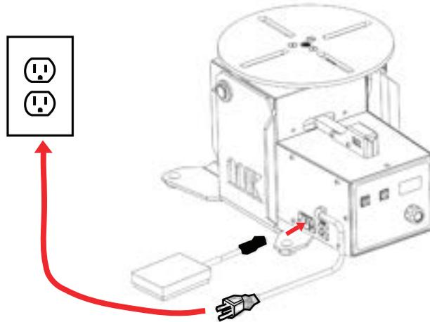
3. If you desire to use the provided foot pedal, plug the pedal cable into connector on the side of the unit.
