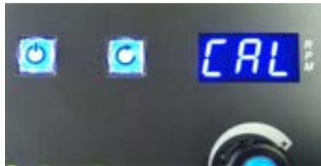
5. Begin the calibration by pressing the start button (knob / push button). Calibration will take about 20 minutes as the table turns and records RPM and time data.
