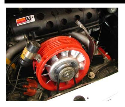
Remove old strap. We recommend cutting off one end to make it easier to pull out from the bottom of fan housing.
