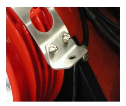
Attach end brackets using the supplied stainless steel hardware.
