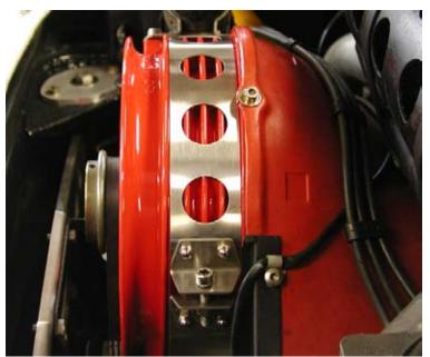
Install tension allen bolt/nut and tighten.
