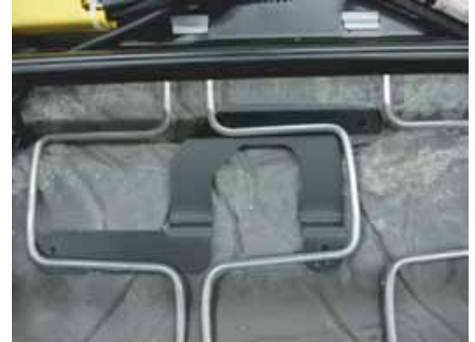
Step 2 - Place the black mounting bracket between the seat springs and seat cushion as shown in the above photos. Slide the bracket up toward the front of the seat until the holes line up with the factory holes shown in step 3. To make this step easier wedge something between the cushion and springs to give you clearance to position the bracket.
