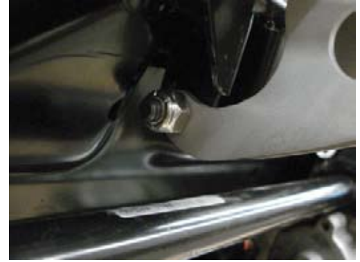
Step 2 - Attach the S/S bracket to the seat as shown in the photos above using the 1/4-20 shoulder bolt and nut. For cars that already have a bolt in this location, remove factory bolt and use the one supplied with this mount.
