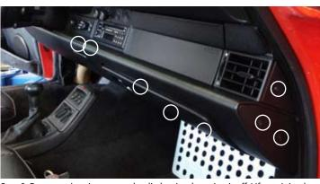
Step 3: Remove trim piece around radio by simply prying it off. Lift retaining bar
