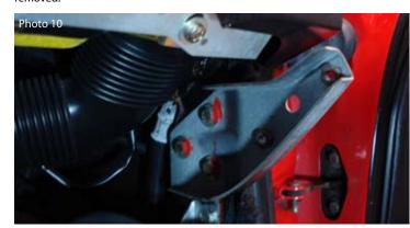
Step 12: Using the (2) supplied .5" button head screws, nuts and washers attach the bottom of the dash panel into the factory holes on the drivers side and center of the dash.
