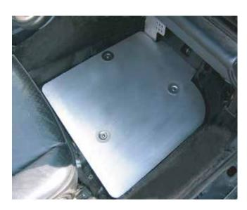
Remove track mat and use supplied riv nut tool to install the riv nuts and then install the embossed washers using he supplied M6 Hardware.
