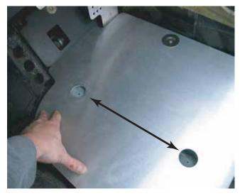
Install Track Mat into car and attach Track Mat to the mounting bracket. Drill 3/8" holes into frame rail in the center of the Track Mat mounting holes.
