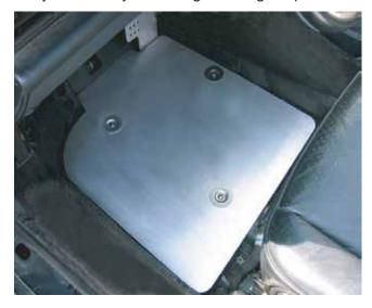
Remove track mat and use supplied riv nut tool to install the riv nuts. Install the track mat using the embossed washers with the supplied M6 Hardware.
