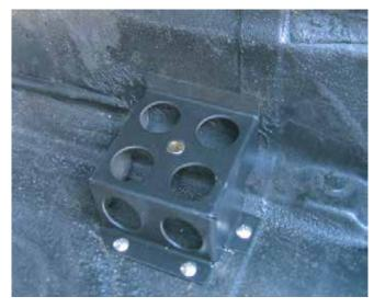
Attach mounting bracket to the floor of car in the desired position. NOTE: This unit can be installed in several different ways. We supply screws and nuts for mounting through the floor pan. If you are welding or drilling into the tunnel of the car, check for hoses, lines or any other object that may be damaged during the process.
