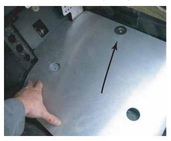
Attach mounting bracket to the Track Mat using the supplied M6 Machine screw and embossed washer. Position Track Mat into car and mark location for mounting bracket.
