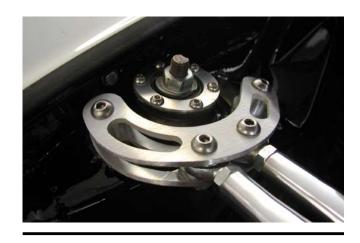
Install as shown above. Note: Drivers side top bracket is marked with a red dot on the top side Keep all bolts finger tight until installation is complete.
