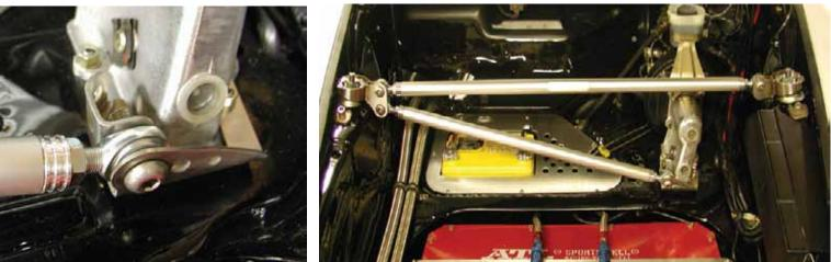
1. If you are installing this brace on a RHD car, reverse the brackets in step 1&2.
