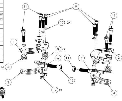
Install as shown Above Note: Strut mount brackets are marked with A,B,C,D to note their location Keep all bolts finger tight until installation is complete.
