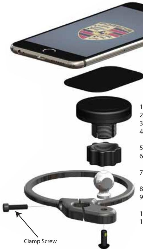
1. Install the aluminum ball onto the metal bracket as shown using the supplied screw.
