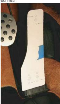
Cut out the supplied template and place over the top of the factory pedal in the desired position and attach with tape. Using a 1/16" drill bit, drill the (3) larger holes that are marked with an X.
