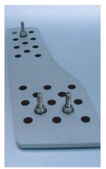
Install the (3) S/S oval head screws, washers and nuts as shown in the photo. Do not tighten screws. NOTE: If you are installing a throttle extension, install extension plate between the pedal cover and washers.
