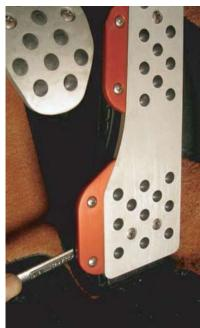
Lock pedal cover into desired position by tightening the (3) nuts on the back of the pedal cover using a 3/8" wrench. Press pedal several times to insure that there is no interference with carpet or any other objects in the pedal
