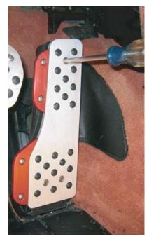
Attach the pedal cover assembly to the lifter plate as shown. NOTE: Make sure that all screws are started prior to adjusting. Adjust pedal to desired height and angle by tightening or loosening the (3) oval head screws.
