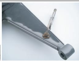
Step 1 - Remove engine mount from engine and thoroughly clean using a degreaser.
