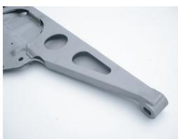
Step 6 - After welding is complete, sandblast entire unit taking extra caution not to remove paint between gusset and factory mount. Grind any welds or imperfections
