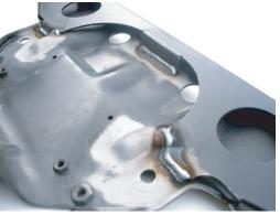
Step 5 - Once unit is all together, execute final welds to all seams that make contact with the factory mount. We stitch weld our long seams (see step 4 photo). Feel free to do complete welds if desired.
