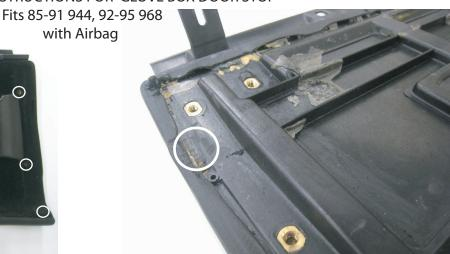
Step 3. Carefully grind or cut away remnants of factory stop arms from outside cover on both sides.
