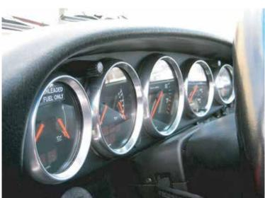
Thoroughly clean factory bezels removing any contaminates such as Armor All that may inhibit the tape to properly adhere to the surface. Remove the backing from the applied tape and install the aluminum bezels over the top of the factory bezels. To insure proper adhesion of the tape, apply equal pressure to all sides of the bezels. Note: This is an acrylic based tape, full adhesion will not be achieved for a few days after installation.
