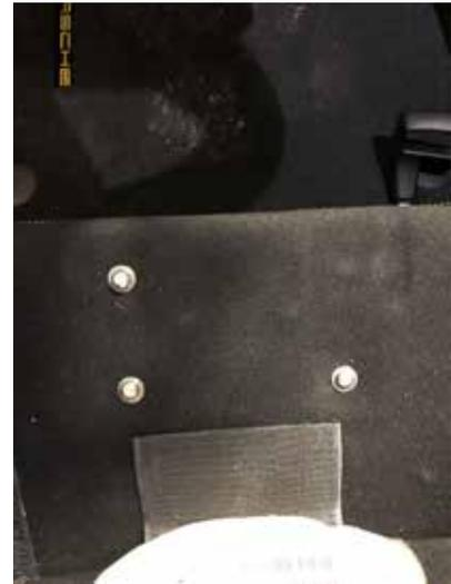
Step 3: Install Rennline Fire extinguisher mount using the supplied M8 nuts and washers. Reinstall wire terminal with integrated nut.
