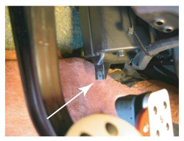
Locate mounting tab on the bottom left corner of the fresh air housing. Insert the supplied speed nut on to tab.
