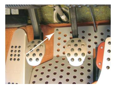
Position floorboard so that the bottom edge is parallel to the floor. Using a 1/8" drill bit, drill a hole through the carpet and into the chassis of the car. Attach floorboard using the supplied sheet metal screw.
