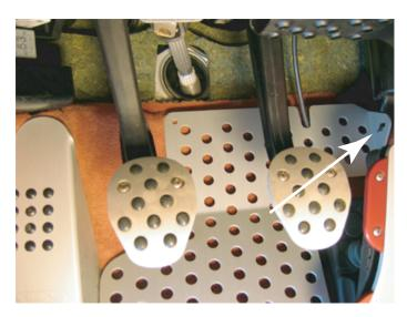
Place floorboard into position and attach to speed nut using supplied sheet metal screw.
