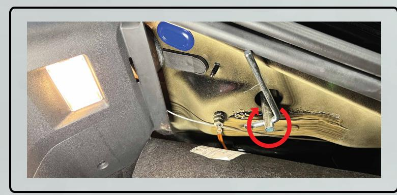
10. Transfer the headlight removal tool to the passenger side, grab your passenger side Morimoto headlight, bring it to the car and plug in the DRL harness. Next line up the guide pins on the sides of the headlight with the channels on the vehicle and slide the headlight into it's place. With one hand turn the tool counter clockwise while pressing the headlight into the fender with the other hand. Carefully turn the tool til you hear a pop sound.
