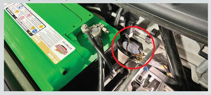
12. If you choose the #1 grommet location then route the Fuse Tap Harness through the grommet (try and keep the opening minimal so you dont have water leaking into your car). From inside the car, pull back the sound deadening material circled below. Then route the harness either below the pedals and behind the sound deadening material (#1) or above the pedals (#2).
