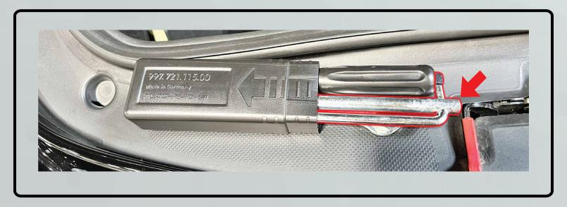
4. Starting on the passenger headlight, insert the headlight removal tool into the hole that had the rubber plug. Note that inserting the headlight removal tool might take a few tries for it to seat on the bolt head. With the tool corretly seated, rotate the tool clockwise approximately 90 degrees til the headlight pops forward. Then simply slide the headlight forward away from the car and set the headlight to the side.
