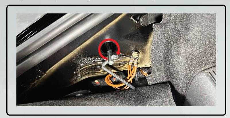
5. On the driver side headlight, insert the headlight removal tool. Rotate the tool counter clockwise about 90 degrees til the headlight pops forward. Then simply slide the headlight forward away from the car and set the headlight to the side.
