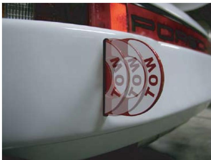
Cut a slot into bumper allowing tow hook to be extracted without rubbing on tow hook finish.
