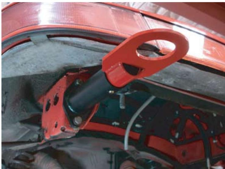
Mount the tow hook assembly into the factory bumper shock location using the factory shock flange and hardware on all 1989-1998. Porsche 964/993. If this assembly is being used for a custom application, other brackets and fabrication may be required.
