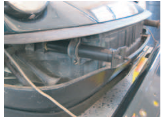
Step 6 - Install Rennline bumper shock. Note: On some early cars, the rear mounting hole is a smaller size than required. Ream hole to the appropriate size.
