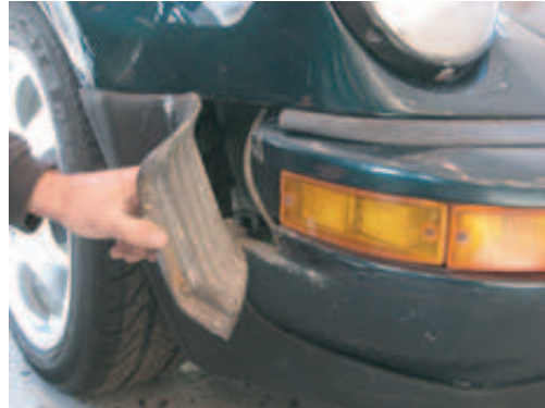
Step 2 - Disconnect one half of side bellows on both sides of car.
