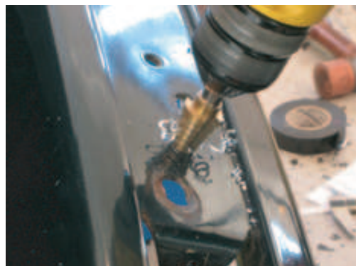
Step 8 - Drill a 3/4" hole into bumper. We recommend using a step drill for the process.
