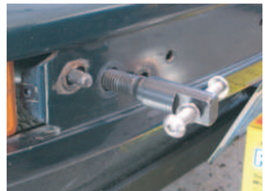
Step 9 - Place bumper onto car and check hole placement by inserting tow hook screw. Make adjustments as needed.
