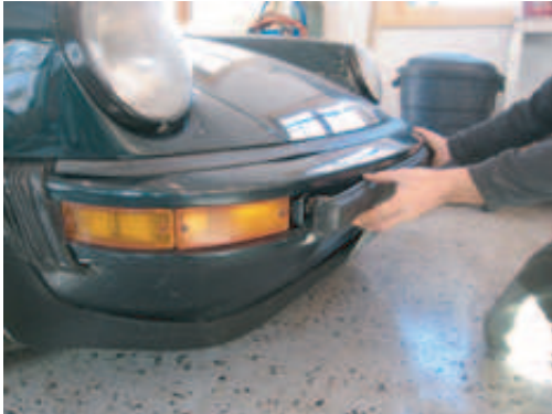
Step 1 - Remove front impact strip.
