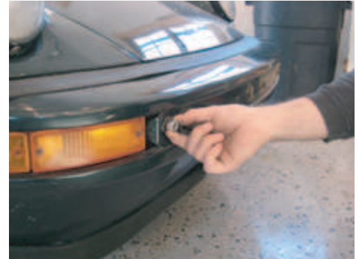
Step 3 - Remove (4) bumper bolts.
