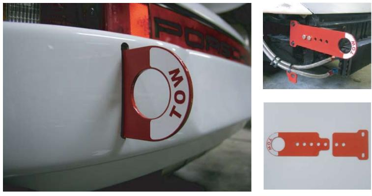
Mounts to factory bumper shock attachment point on all 1974-1989 911's using factory hardware. Although this is a bolt on unit for 911 based cars it can be used for several custom applications.
