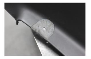
30. Drill hole out with 1 7/8" hole saw. Clean up the cut out with a rotary flap sander.
