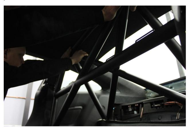
23. Align interlock connections and start all allen bolts (1/4" allen head). A tapered drift tool works best to align holes.
