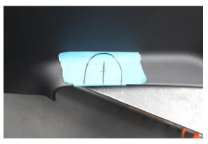
29. Drill pilot hole. With exacto knife cut out shape in the vinyl layer and peel off
