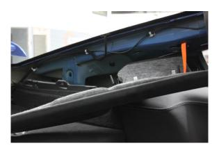
9. B pillar seat belt trim pulls out from the top first then lift up. The rest of the B pillar trim piece pulls straight out to the middle of car. There is a lock tab that is difficult to release without a right angle pick tool. It can be accessed through a hole in the body with some careful maneuvering.
