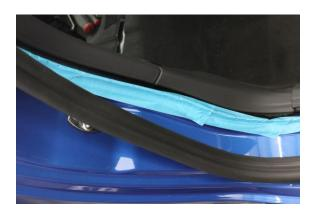
11. The door sill trims can be pulled straight up. Unplug connector on driver side.
