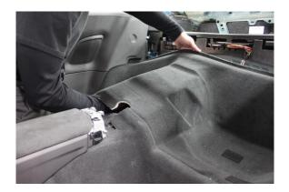
13. Place some tape over the lower flat area of the rear side panels. Mark the center line of the lateral beam below carpet onto the tape for both panels. This will be your reference for making the holes for the main hoop.
