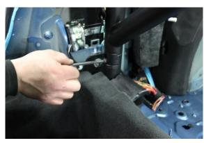
24. Make sure the rear mount bolts can be started. Tighten the allen bolts then the 3 bolts at each base mount.
