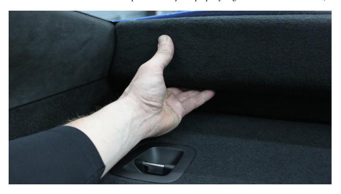
6. The upper rear carpet shelf can now be removed by first prying off the tie down point trim, then pull the piece up from the middle allowing it to fold up and out.
