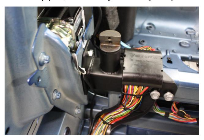
20. Be sure no wires are pinched by new base mount on sides of car. Using pliers or a knife, break off tabs on bottom of wiring harness guides to allow for a tighter fit.
