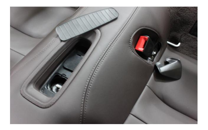
4. (GT3 skip this step) Remove rear seat back rests by first removing the back half of the center pivot point trim. This piece pulls straight up. The front half can then be worked off from side to side towards the front of the car. The seat backs now slide into the center of the car then can be pulled up & out.
