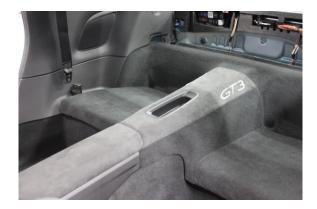
34. Cut off raised lip of carpet as shown in picture for easier installation of bar. (Do this on both sides. This will not be visible after complete assembly).
