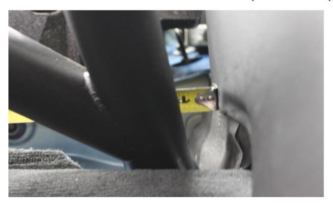
41. Draw out an oval that is approximately 1 3/4" by 3" based off of the location measurements.
