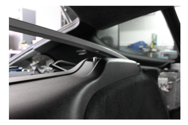
9. Using light stick blue tape (preferable) cover front bulkhead carpet in areas that will need to be cut. Layout the template for this carpet by aligning with the top center and side trim pieces. Make your marks onto the taped areas.
