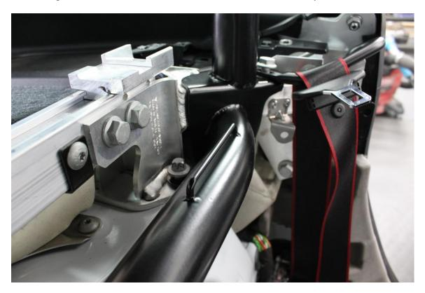
16. Set rear stay bars in place by coming from the front, locate the front strut bolt into bracket first then rotate and tilt into place locating back strut bolt into bracket. Start the strut mount nuts but do not tighten.
