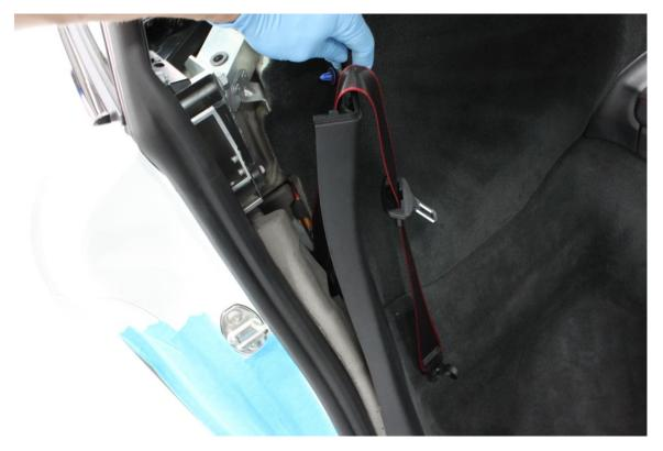
12. The top center trim can now be removed by pulling it straight up. Now the front bulkhead carpet can be lifted out.
