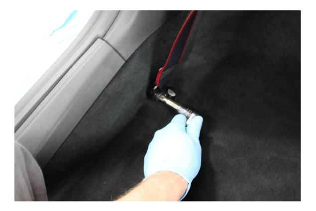
7. Take off the top corner trim where the seat belt comes out of by pulling out and up working your way around the piece. After piece is loose the seat belt can be pulled through the opening.
