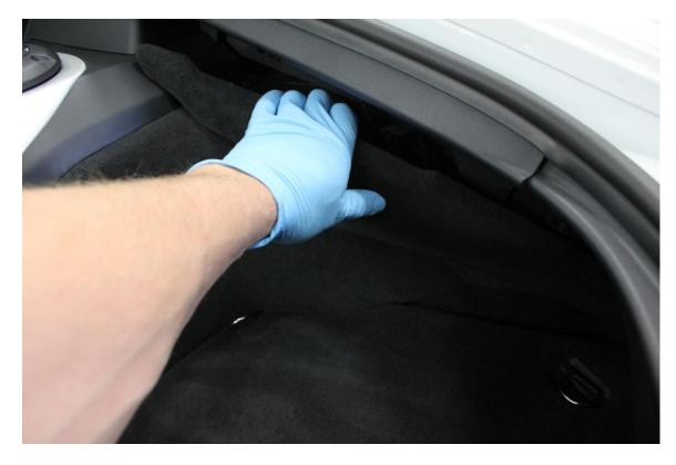
2. Twist off the two fluid access covers on the rear center garnish. Then pull out the strut cover trim pieces by pulling them into the center of the car. Remove the two outside 13mm nuts from the top of the strut mount.
