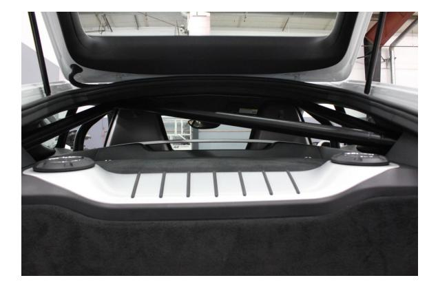
1. Remove rear carpet side pieces by grabbing in the upper gap and pulling to center of car.
