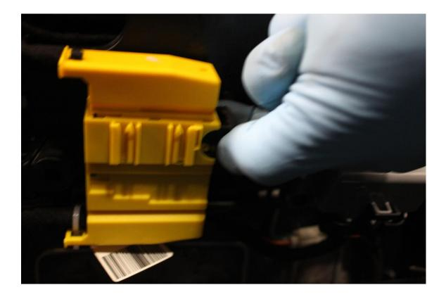
6. Unbolt the factory seat belts at the bottom bolt on car by flipping the cover cap open first. After bolt is out, remove the bolt cap/cover assembly from the seat belt lower bracket so that the seat belt will slide out of the top trim piece later.
