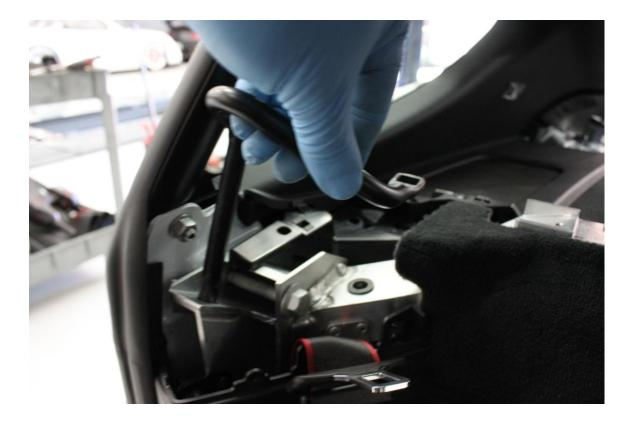
11. Pull up lower door sill trim. Then remove the side trim pieces by pulling the tops of them into the car then lifting up and out.
