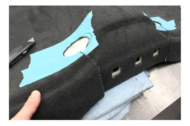
15. Two people make the carpet/hoop install easier to manage. Bring cut carpet piece and hoop assembly into the car. Set hoop loosely in place. Begin to fit carpet piece around the center of the harness bar. Now set carpet and hoop in place together. Start bolts to bulkhead brace then refit seat belt guides with bolts. Keep bolts loose to allow bar to be rocked a little for assembly.
