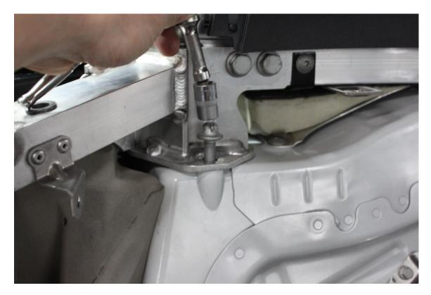
14. Begin cutting the bulkhead carpet holes out. Following the pictures, notice where the foam on the back side needs to be removed for clearance. The top corners of the carpet piece will need to be cut off for the main hoop base. Also notice where the additional slits will need to be made for the main hoop lower plate and the center holes for installation around the harness bar.
