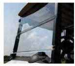
Acrylic Windshields for ST cars with short tops. Come with the original rubber mounting clips.
