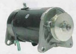
Starter Generator, Yamaha 4 Cycle Gas G2-G14 OEM: J38-81100-10; J38-81100-11,
