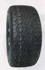
Mojave Steel Belted Radial 23x10.5R12 SBR DOT, 6 ply. TIR-395
