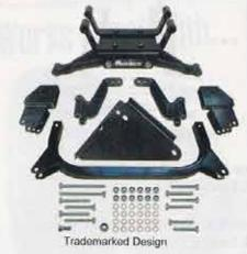
BMF 6" A-Arm Lift Kit, Yamaha G22 Gas and Electric LIFT-504
