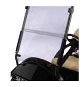
Acrylic windshield. Includes mounting hardware and gasket at bottom.
