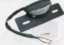
Universal Illuminated License Plate Holder License Plate Holder with LED Plate Tag Running and Brake Light, 12V
