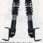
Two mounting holes and threaded body allow for extra camber adjustment. Sold in a set of 2.
