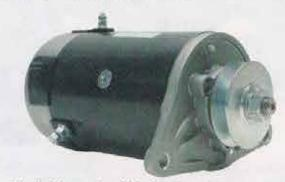
Starter Generator, Club Car Gas 84-96.5. Counterclockwise Rotation (Non-Subaru) OEM: Can also be wired for clockwise rotation (Precedent and DS 97+). OEM: 1012316; 1018294-01, 1018294-99; 1018337-01.
