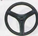
ACC-SW158 Brenta ST Steering Wheel with Carbon Fiber Insert
