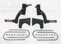
6" Drop Spindle Lift Kit, E-Z-Go TXT Gas 08.5-19 with Kawasaki Engine LIFT-110
