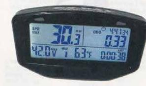
Digital speedometer with waterproof connections features non-resettable odometer, average/max speed, air and motor temperature (ACC-0200 only), battery voltage readout for electric golf cars, alternator battery health for gas golf cars, programmable maintenance reminders, ride time, total accumulated ride time, LED warning lights and auto On/Off.
