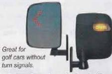
LED Side Mirror Set with Running/Turn Signal Light Capability, 12-48V, 3 Wire
