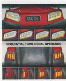
Light Kit features sequential turn signal operation on both headlights and taillights
