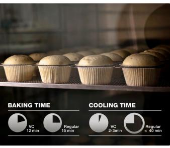
2. As the bread is allowed to finish baking during the vacuum cooling process, the total baking time is reduced with up to 30%. The actual cooling only takes a couple of minutes. Hence the baking and cooling time can be reduced to less than 15 minutes depending on products. This results in energy savings as well as less man hours needed. Also, you'll need less floor space due to fewer racks in the bakery.
