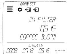
To link the keys to the saved positions, start from the standby visualization and press for 1 second the intended key: the appliance displays the list of saved regulations/positions. Turn the knob for scrolling and press to confirm the link. For the keys with no link, the display shows the following indication: [-.-].
