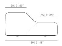
The bench will be provided with the raised part on the right or on the left. Indicate the desired option in the order, remembering that left / right is understood by looking at the element for manufacturing purposes.
