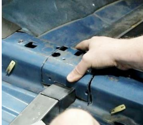
Figure 39 - Fit Seat Riser
