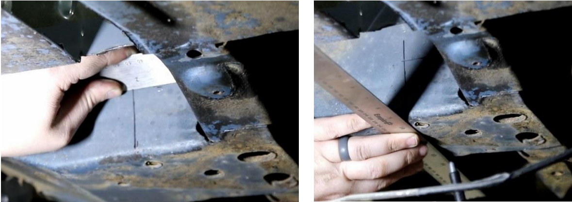
Figure 28 - Project Cut Lines
