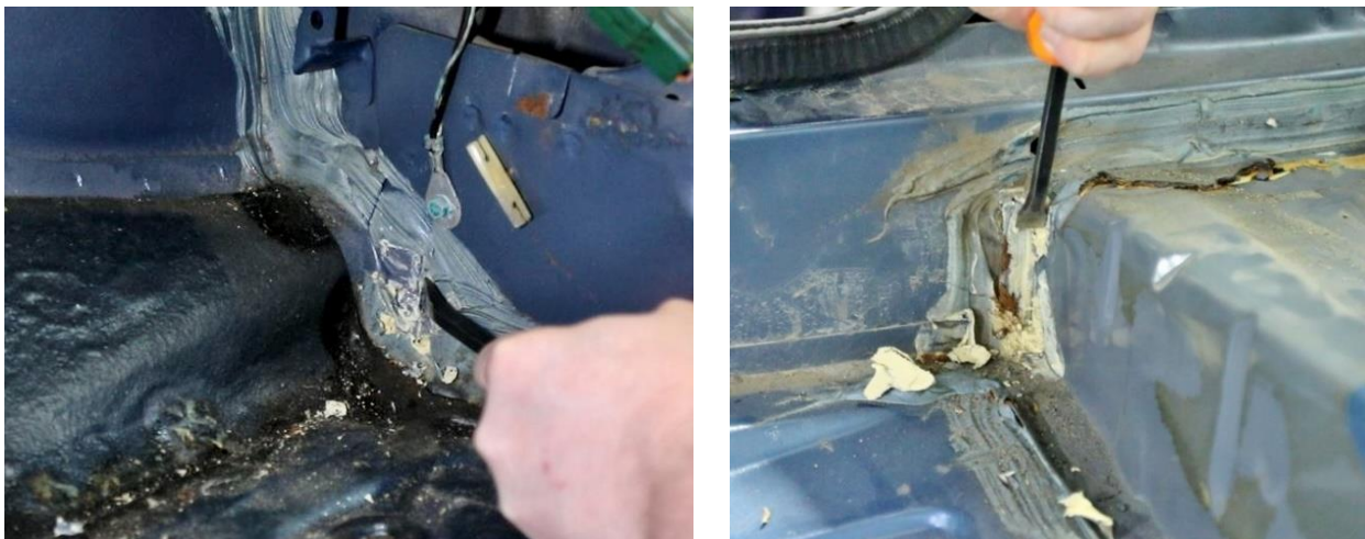
Figure 5 – Remove Seam Sealer
