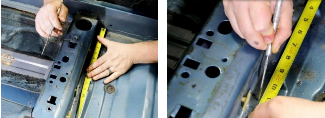
Figure 7 - Mark Seat Riser
