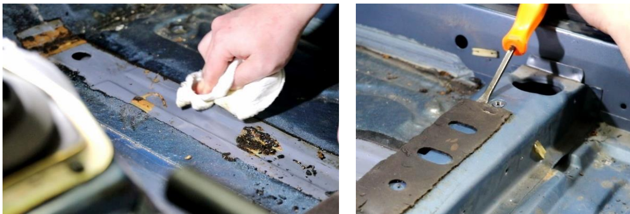
Figure 6 – Clean Cut Area and Remove Foam
