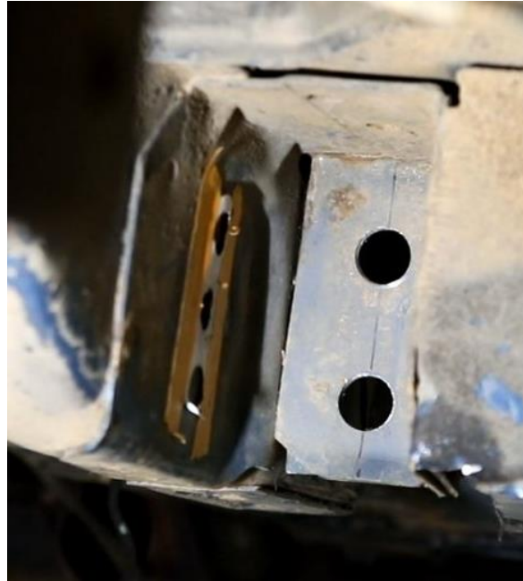
Figure 32 - Drill Plug Weld Holes
