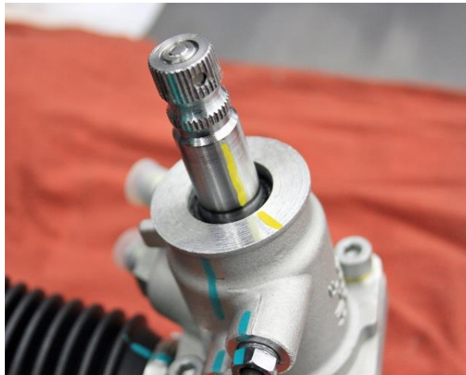
Figure 3 - Center the Rack & Pinion
