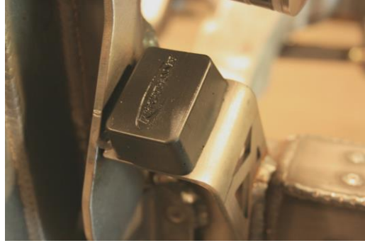
Figure 9 - Installed UCA Bump Stop
