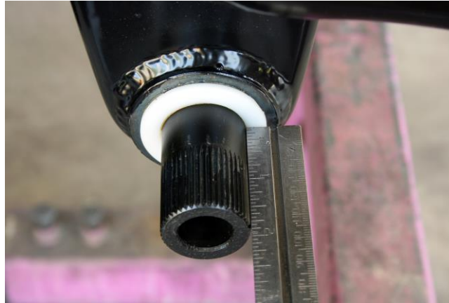
Figure 7 - Measuring the Anti-roll Bar
