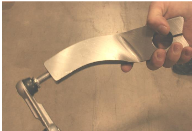
Figure 8 - Pre-assemble the Anti-roll Bar End Links
