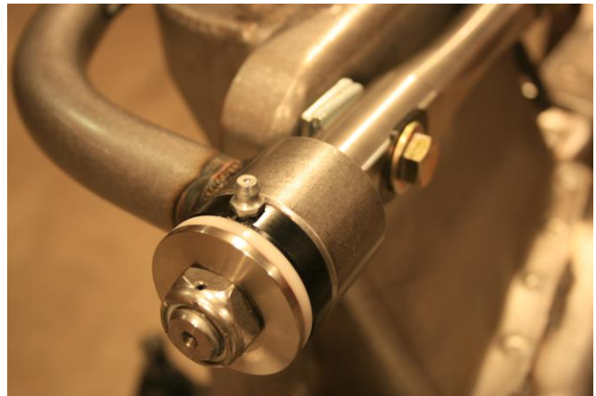
Figure 16 - Installed Upper Control Arm
