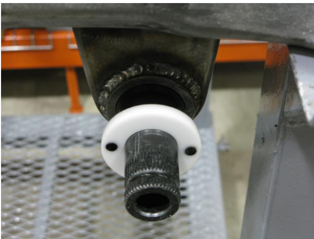
Figure 5 - Installing the Bushing & Anti-Roll Bar
