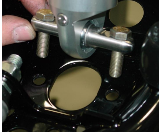
Figure 13 - Lower Shock Retaining Bolts
