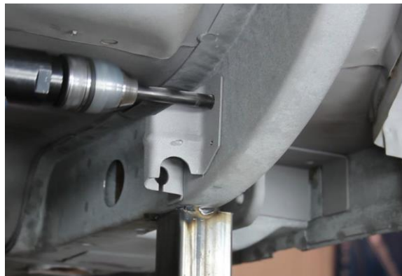
Figure 1 - Remove E-brake Bracket
