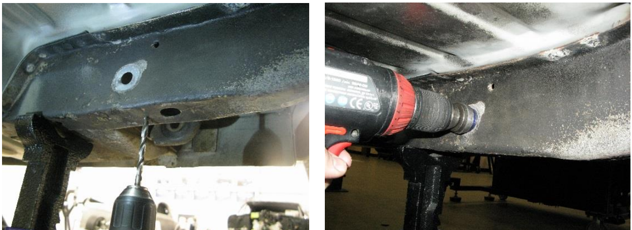
Figure 2 - Remove Factory Crush Tube
