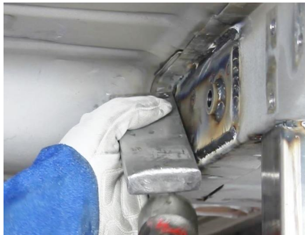
Figure 7 - Modify Floor Pan
