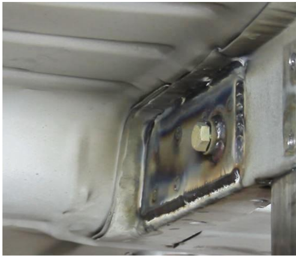
Figure 5 - Weld Outboard Torque Box Plate
