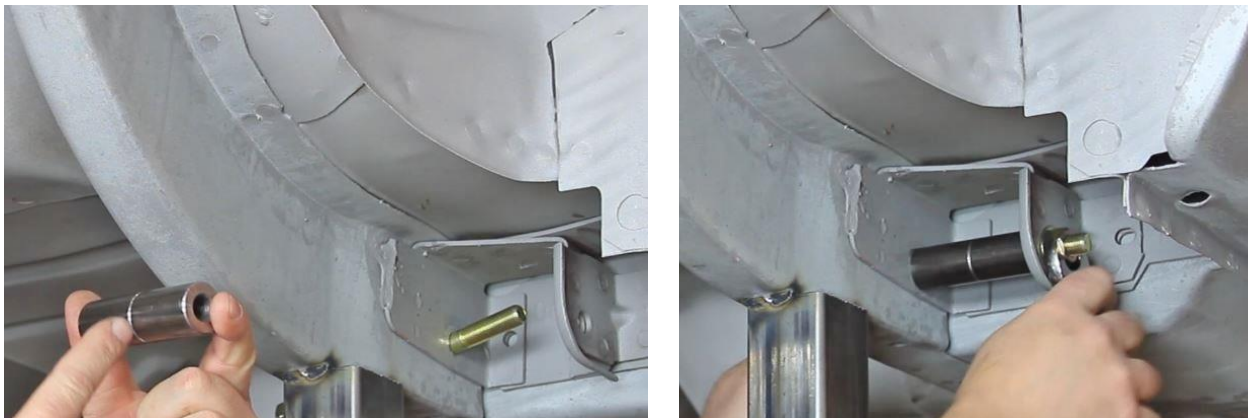
Figure 4 - Install Weld Spacer
