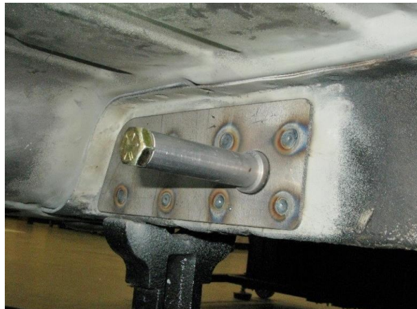
Figure 6 - Install Outboard Torque Box Plate with Stock Suspension
