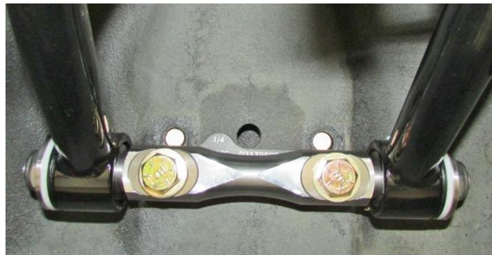
Figure 15 - Install Camber Shims
