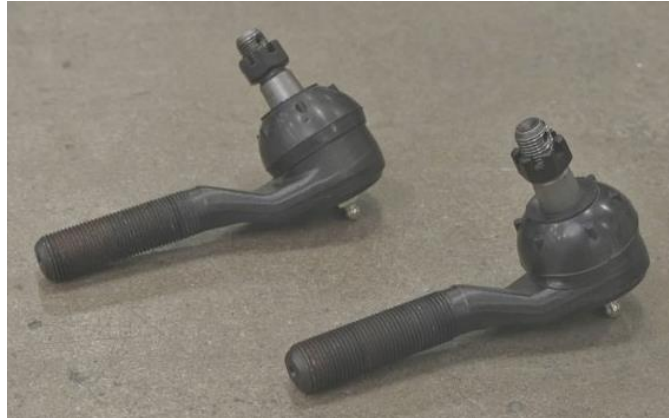
Figure 25 – New Outer Tie Rods
