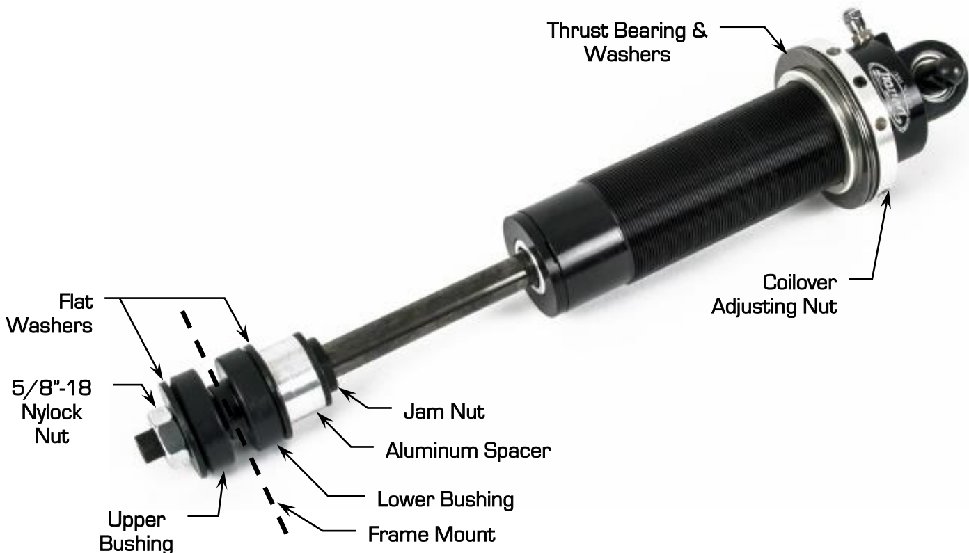
Figure 1 - Shock Assembly
