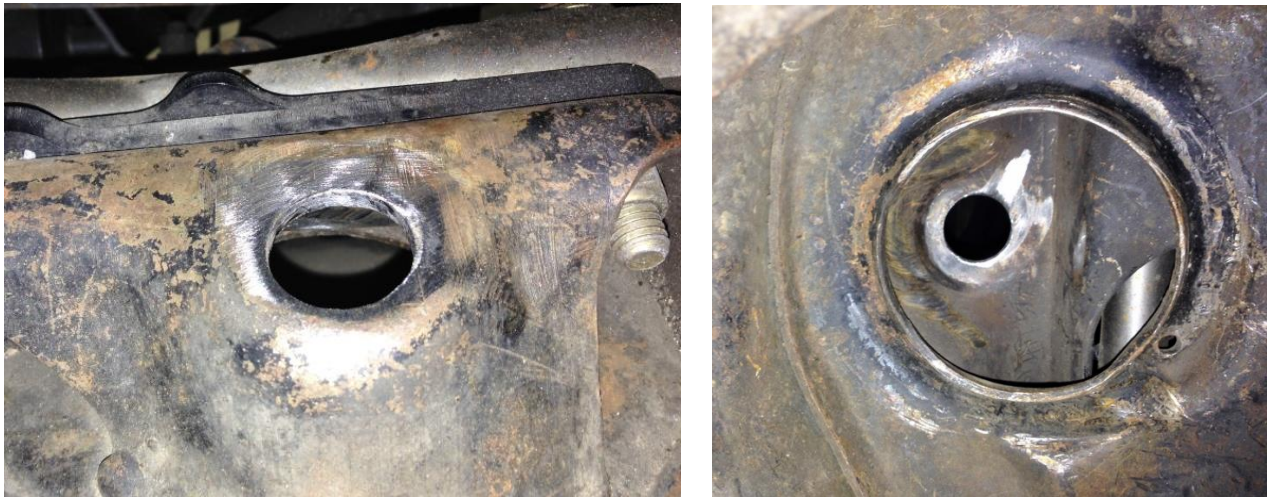
Figure 2 - Remove Sharp Edges/Burrs
