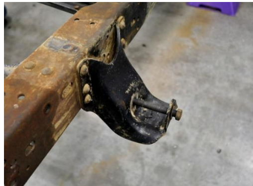
Figure 4 - Rear Leaf Spring Bracket
