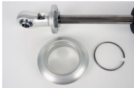
Figure 38 - Upper Spring Seat & Retaining Ring
