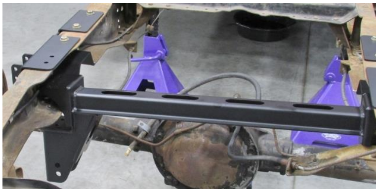
Figure 15 - Position Crossmember Assembly
