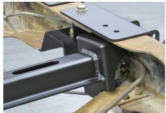
Figure 15 - Position Crossmember Assembly
