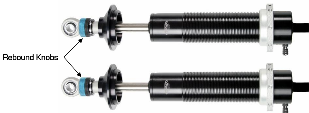
Figure 43a- Detroit Speed Single Adjustable Shock
