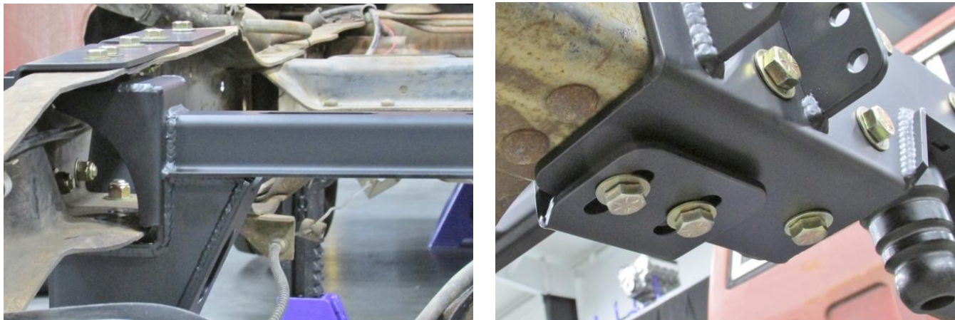
Figure 16 - Install Track Bar Crossmember
