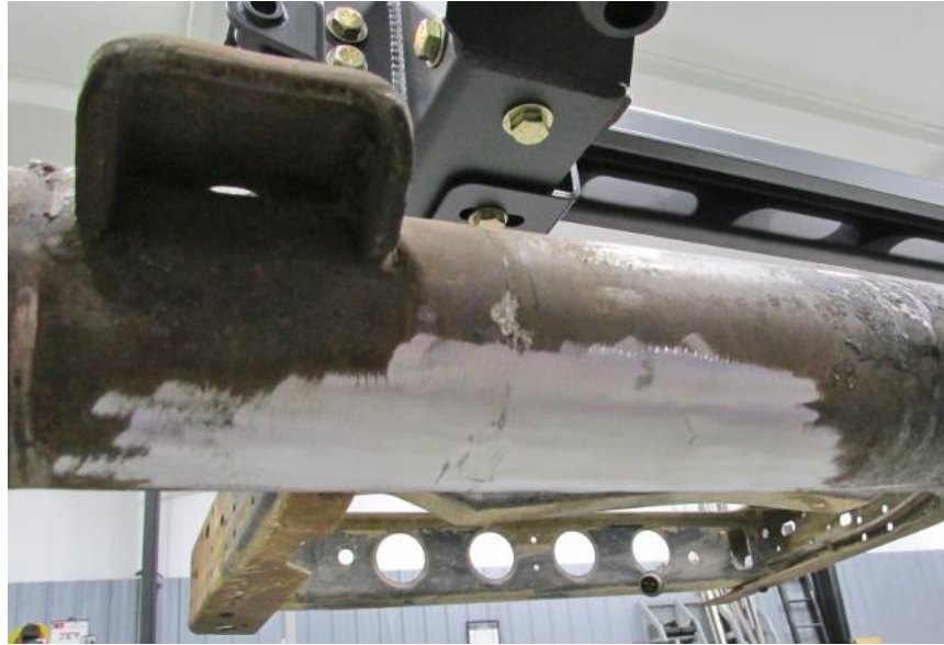
Figure 22 - Cut Off Factory Lower Shock Mount (Passenger Side)
