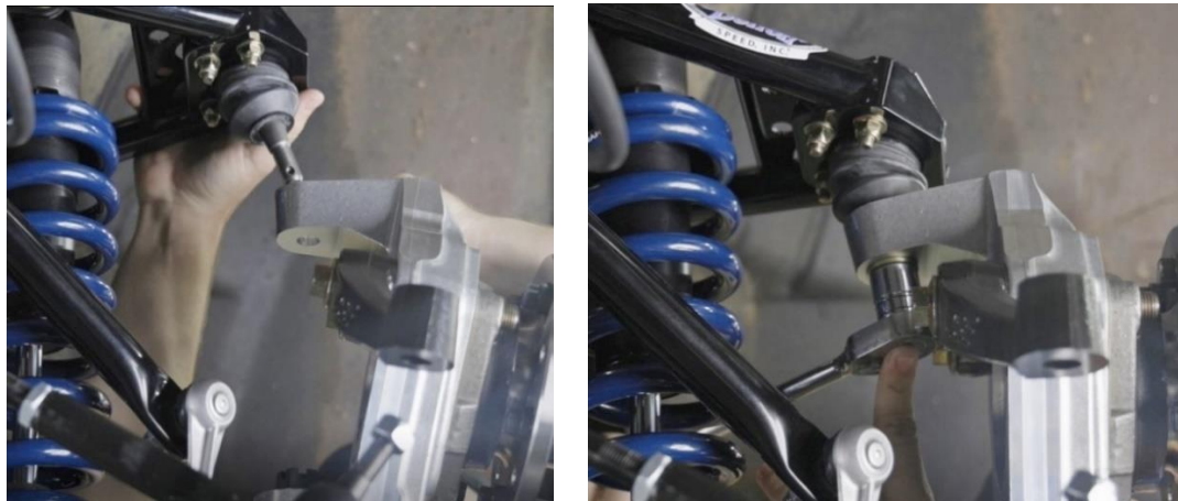
Figure 95 – Install Upper Ball Joint
