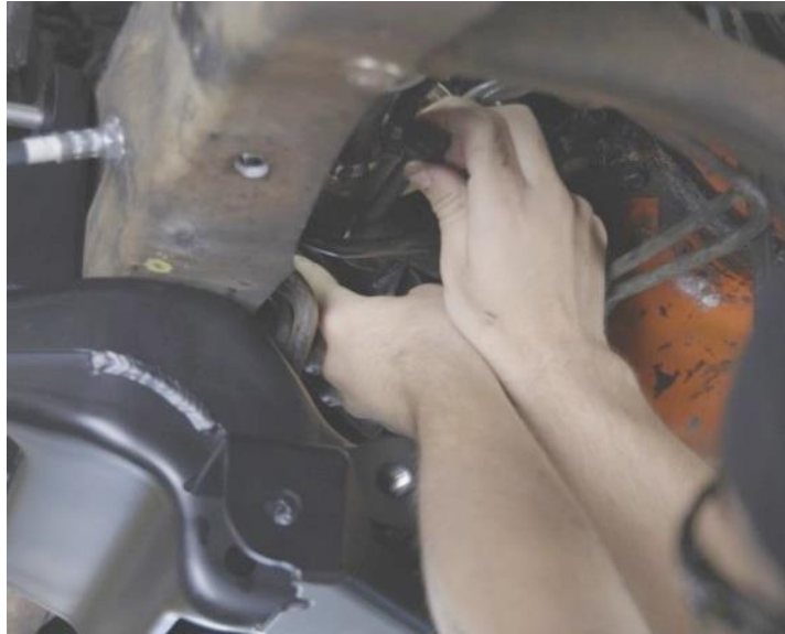
Figure 42 – Install Engine Mounts
