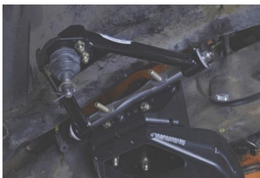
Figure 46 – Install Upper Control Arms
