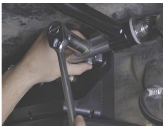
Figure 47 – Install Camber Shims
