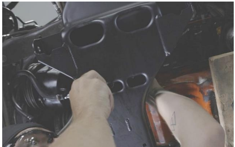
Figure 41 – Install Engine Mount Brackets
