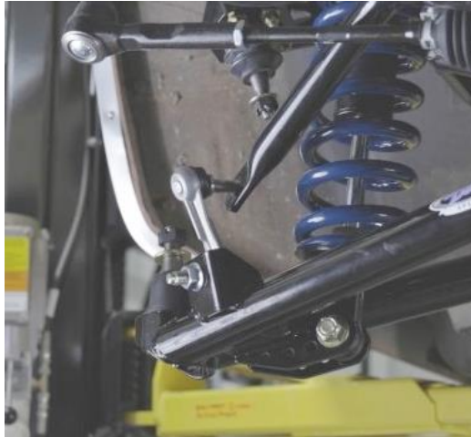
Figure 88 - Install Sway Bar End Link
