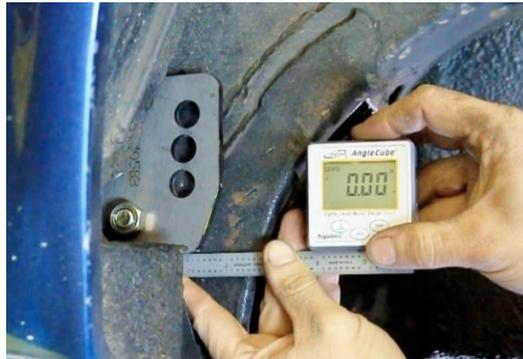
Figure 8 - Level Frame Doubler Plates
