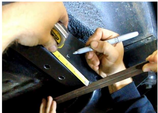
Figure 53 - Locate Access Holes
