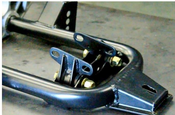
Figure 78 - Lower Differential Bracket Assembly
