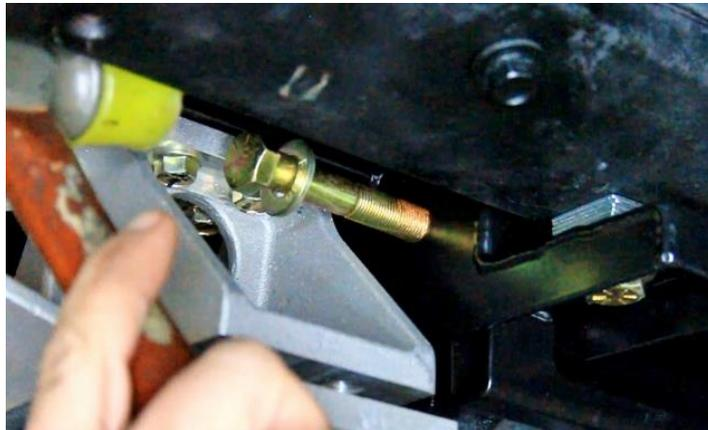
**Figure 89 - Install Differential to Upper Cradle**
