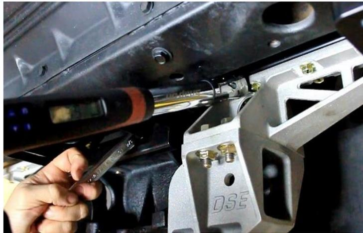
Figure 92 - Torque Upper Differential Bracket
