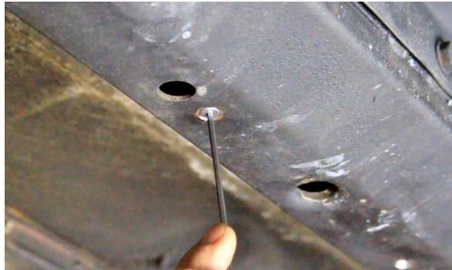
Figure 35 - Drill & Chamfer Holes
