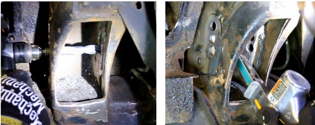
Figure 21 – Drill Upper & Lower Link Holes
