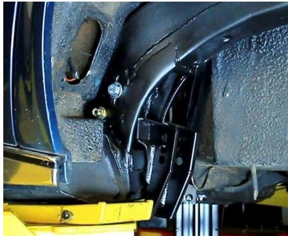
Figure 32 - Install Trailing Link Bracket
