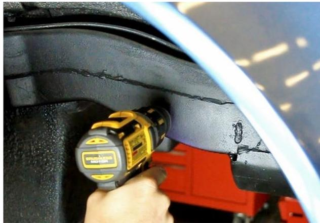
Figure 54 - Drill through Frame Rail
