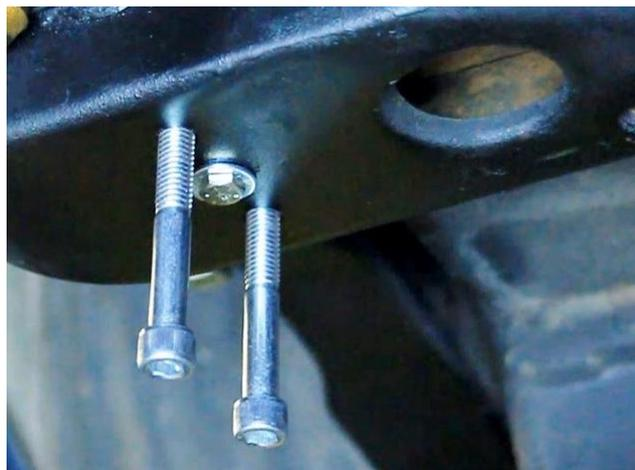
Figure 65 - Install Sway Bracket Nut Plate Assembly
