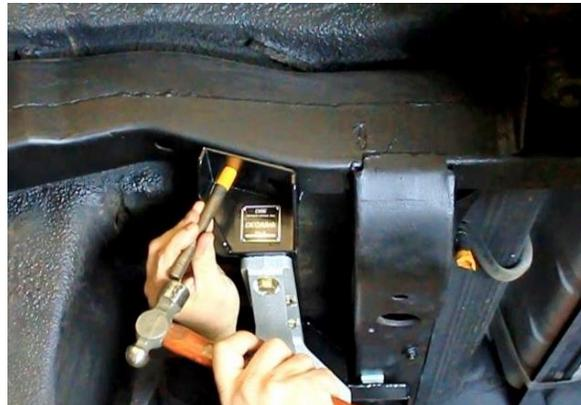
Figure 43 - Transfer Punch Frame for IRS Cradle
