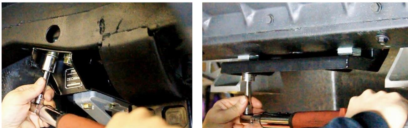
Figure 85 - Torque 1/2"-13 Hardware
