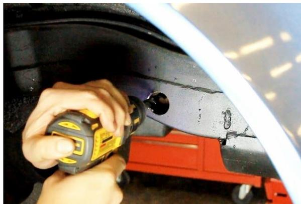
Figure 56 - Drill Inner Mounting Hole
