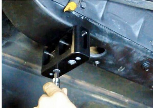
Figure 66 - Install Sway Bracket Spacer
