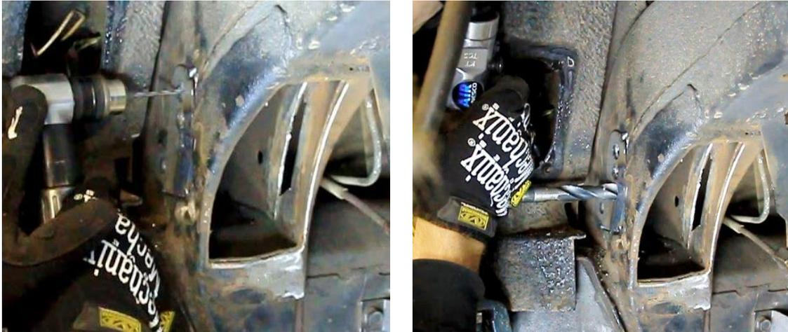
Figure 14 – Drill Trailing Link Holes
