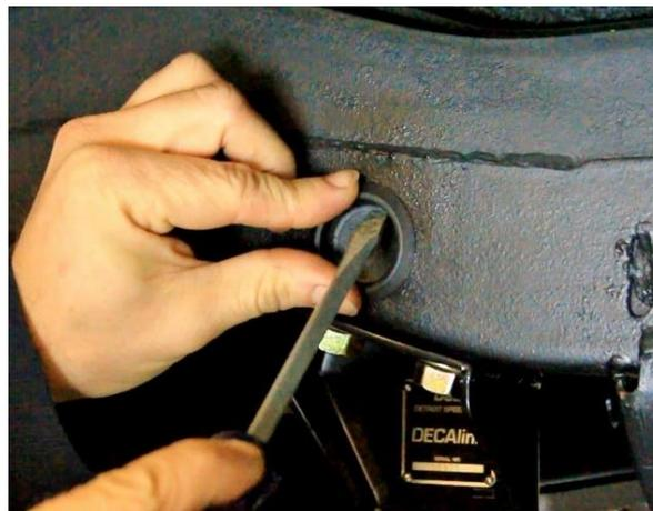
Figure 114 - Install Recessed Plug
