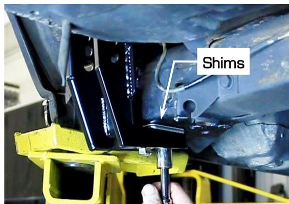
Figure 33 - Install Trailing Arm Bracket Assembly
