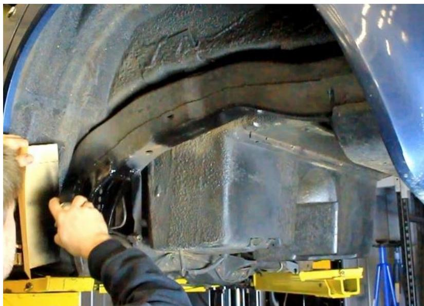
Figure 30 - Paint Modified Frame Rails
