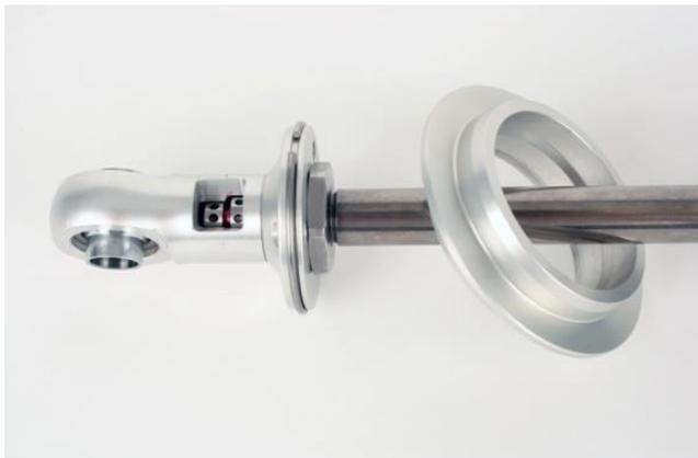
Figure 108 - Removing the Spring Seat
