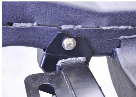
Figure 81 - Install Upper Cradle Assembly to Frame
