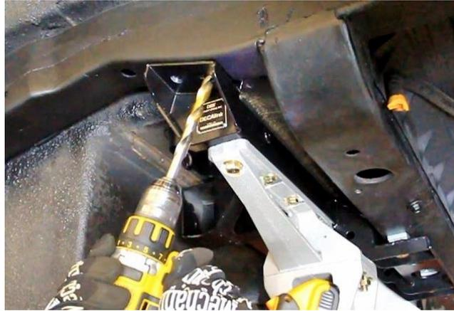
Figure 51 - Drill Bottom Side of Frame
