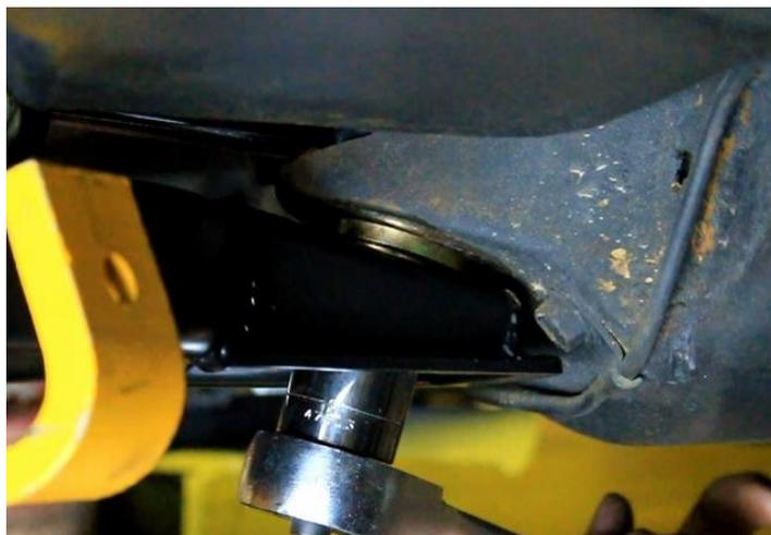
**Figure 90 - Torque Lower Differential Mount**
