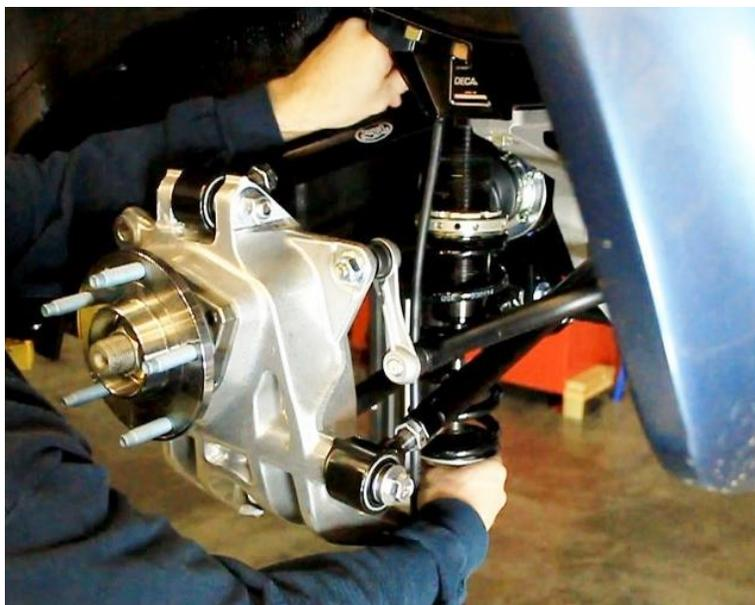
Figure 111 – Install Upper Shock Bolt & Spacer
