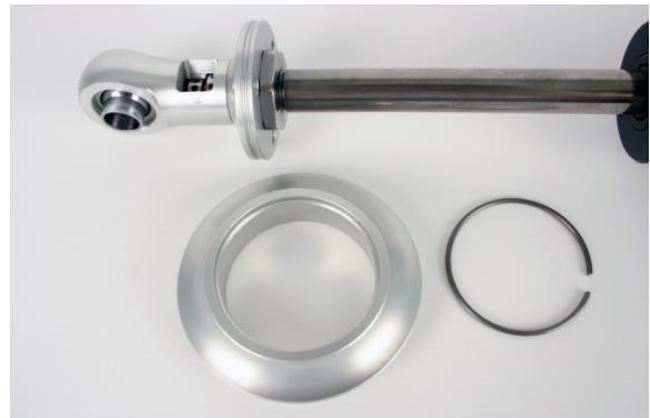
Figure 109 - Spring Seat & Retaining Ring
