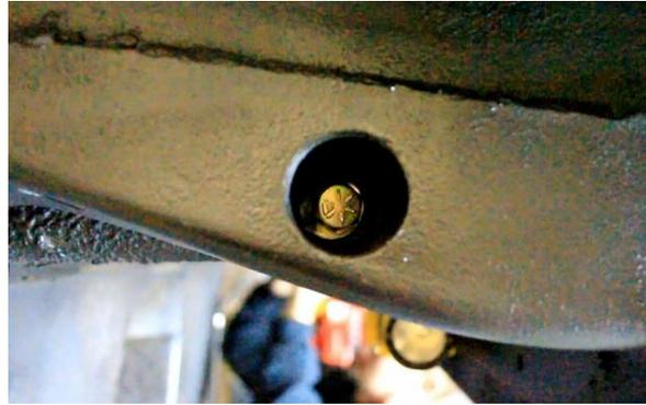
Figure 82 - Install Crossmember Fasteners
