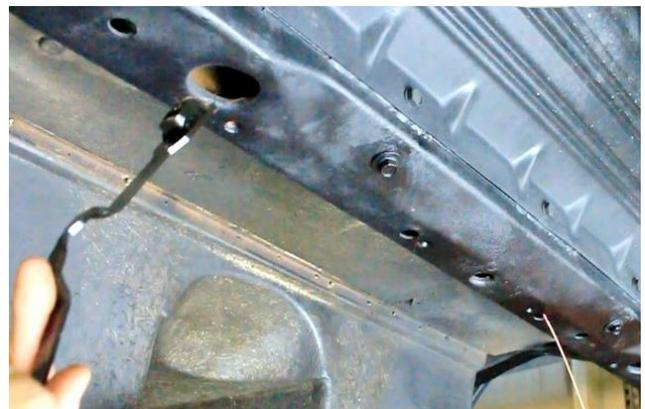
Figure 36 - Bend Crossmember Nut Plate
