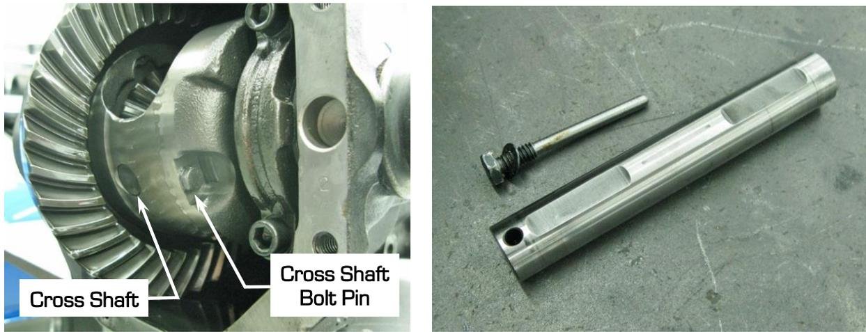
Figure 69 - Cross Shaft & Cross Shaft Bolt Pin
