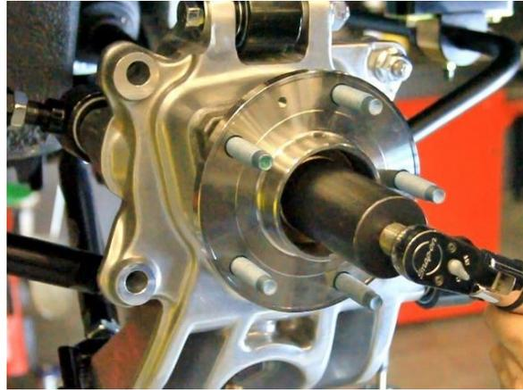
Figure 113 - Torque Outer CV Joint
