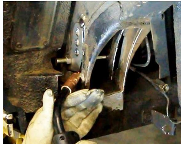
Figure 12 - Tack Weld Doubler Plate
