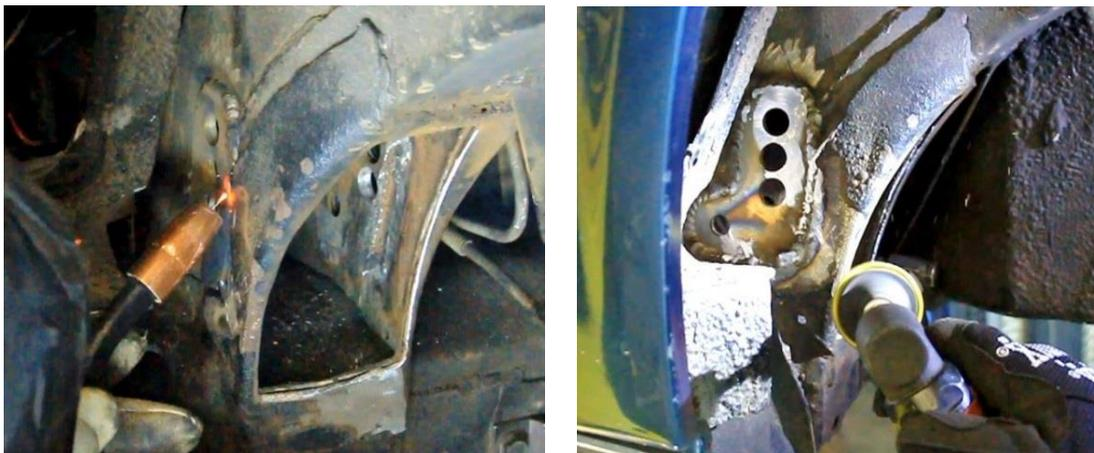
Figure 22 – Finish Weld Doubler Plates
