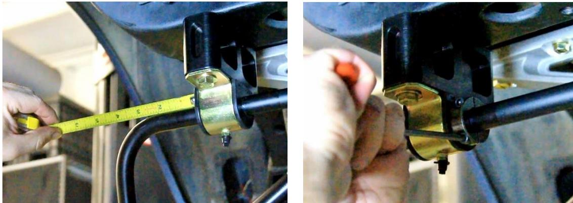
Figure 101 - Center Sway Bar and Install Split Lock Collars
