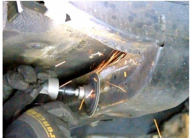
Figure 3 - Remove Frame Crossmember Brackets
