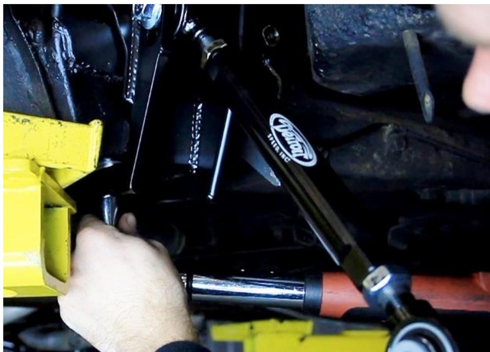
Figure 96 – Trailing Link Bracket
