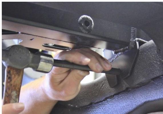
Figure 44 - Transfer Punch Frame for IRS Cradle
