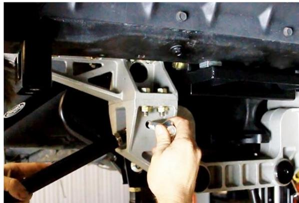
**Figure 99 - Install Toe Link Assemblies**
