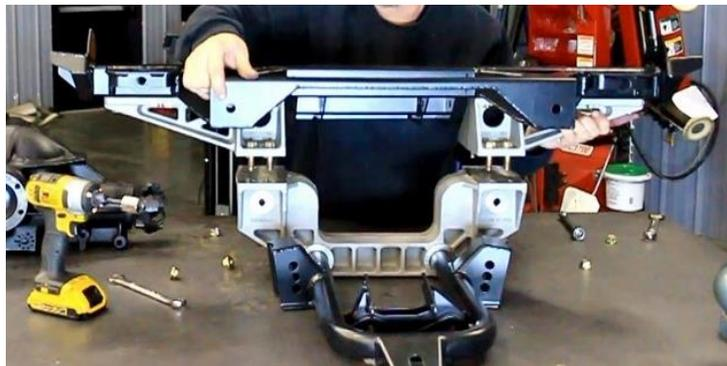
Figure 77 - Disassemble IRS Upper & Lower Cradle
