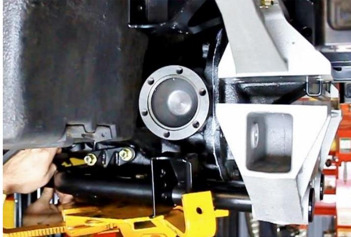
**Figure 88 - Install 5/8"-18 Hardware**
