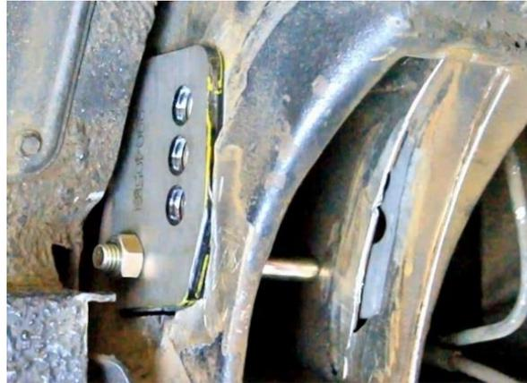
Figure 11 - Verify Frame Rail Modification
