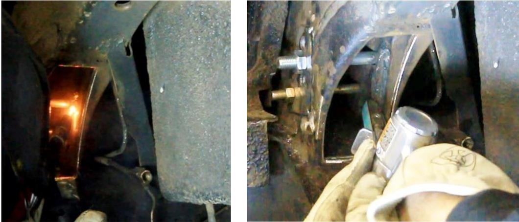
Figure 20 – Weld Inner Frame Rail
