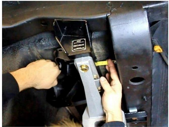
Figure 42 - Level IRS Cradle to the Frame
