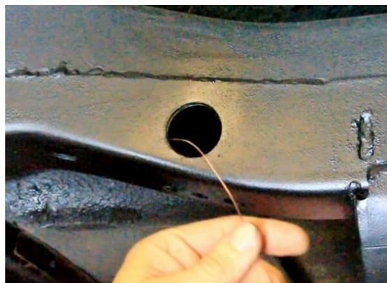
Figure 59 - Locate Lower Cradle Nut Plate
