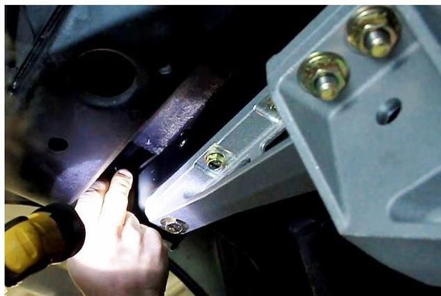
Figure 50 - Scribe Inside Mounting Hole Location
