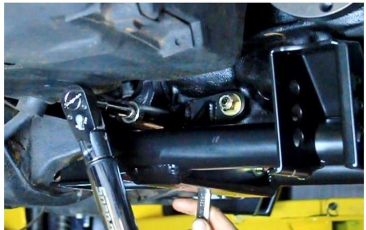
Figure 93 - Torque Lower Differential Bracket
