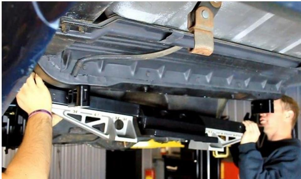
Figure 83 - Install Upper Cradle Assembly to Frame
