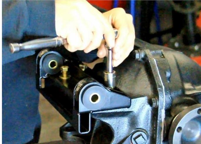
Figure 76 - Upper Differential Bracket Assembly
