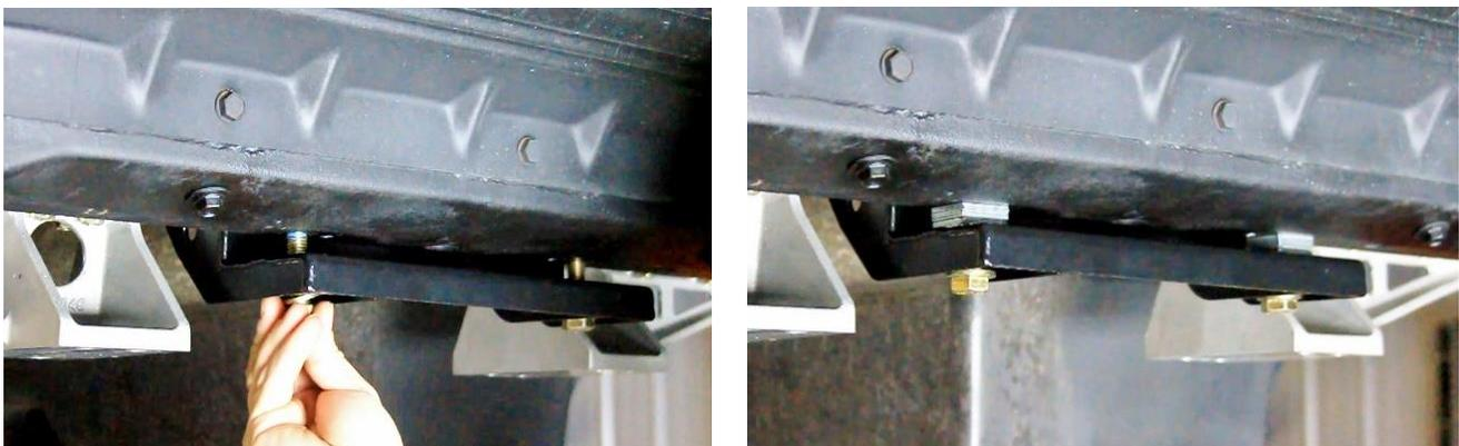
Figure 84 - Install Fasteners & Slotted Shims
