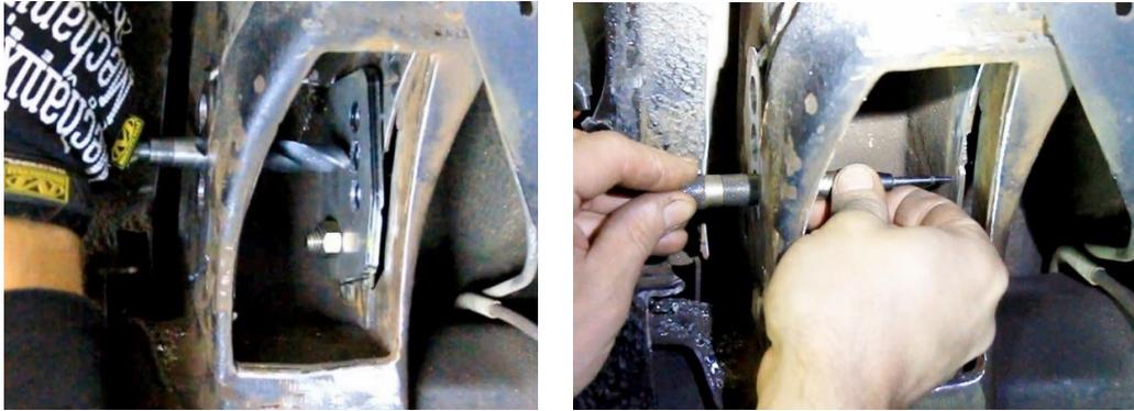
Figure 17 - Center Drill Inner Frame Rail
