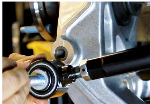
Figure 106 - Install Toe Links
