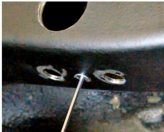
Figure 58 - Drill & Chamfer Nut Plate Locators
