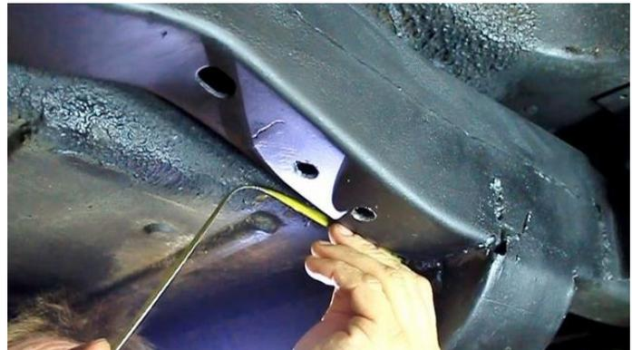
Figure 52 - Locate Inside Mounting Holes
