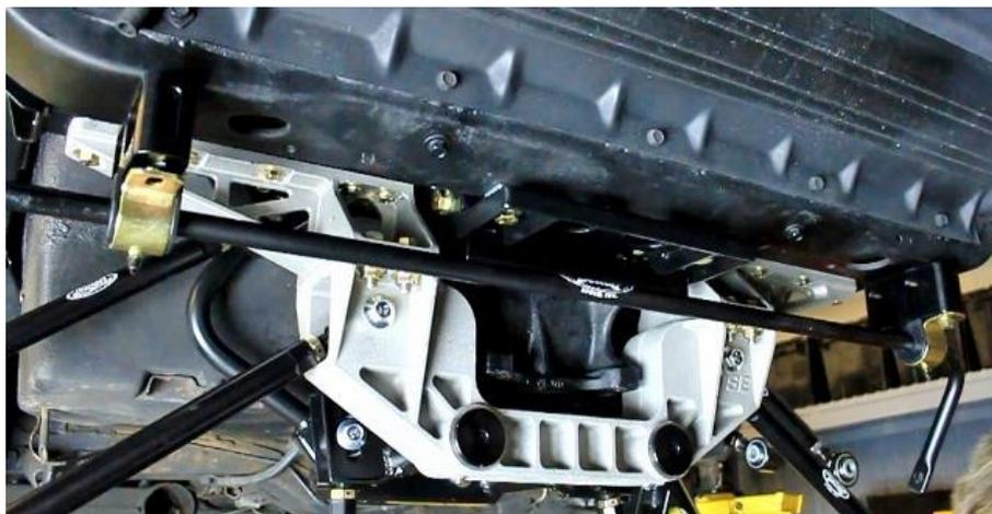
**Figure 100 - Install Sway Bar**
