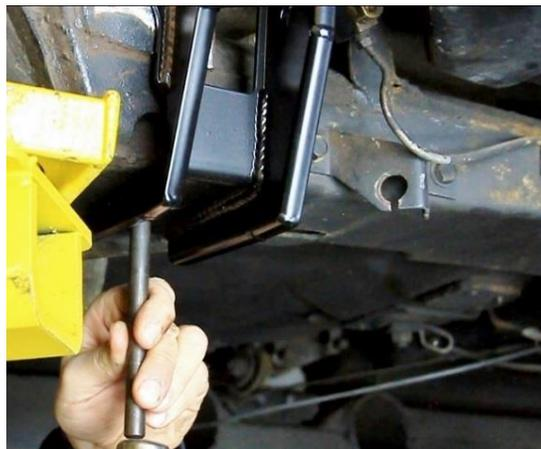
Figure 25 - Transfer Punch & Drill the Frame
