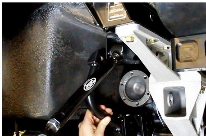
Figure 97 – Install Upper Lateral Link & Tie Braces
