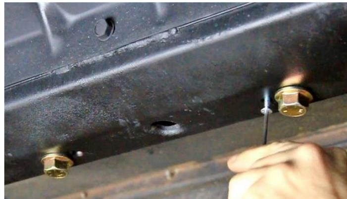
Figure 38 - Install Crossmember Nut Plate
