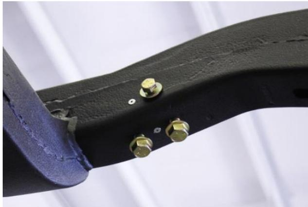
Figure 49 - Install Nut Plate Assemblies
