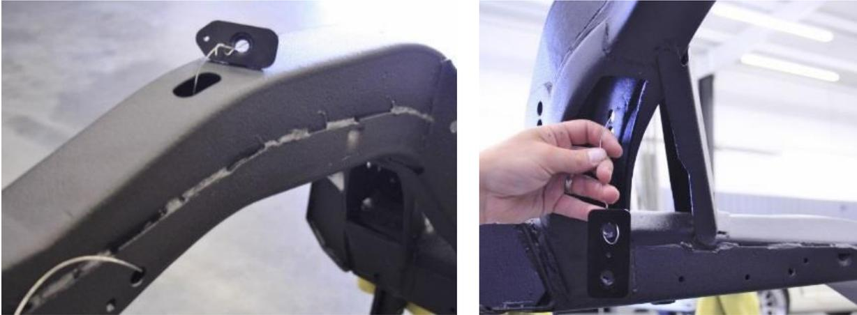
Figure 48 - Position Nut Plate Assemblies
