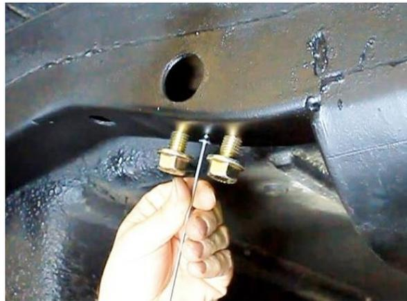
**Figure 60 – Install Nut Plate Assemblies**
