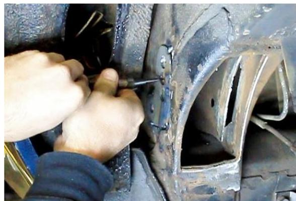
Figure 13 - Center Punch Trailing Link Holes
