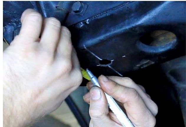
**Figure 61 – Sway Bar Nut Plate Location**
