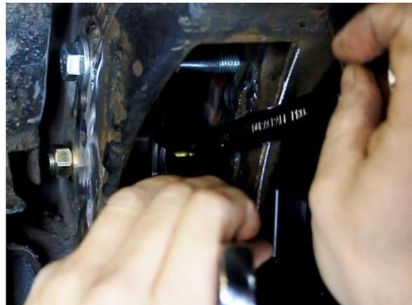
Figure 24 - Expand Crush Sleeve
