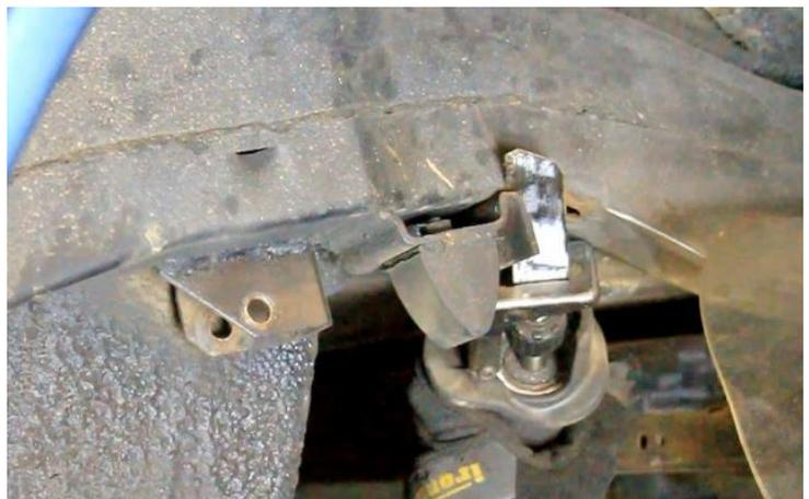
Figure 4 - Remove Frame Bumper and Upper Shock Mount Brackets
