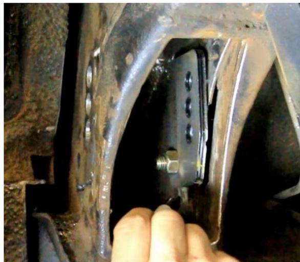
Figure 16 – Level Drill Guide
