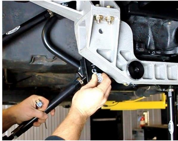
**Figure 98 - Install Lower Lateral Links**
