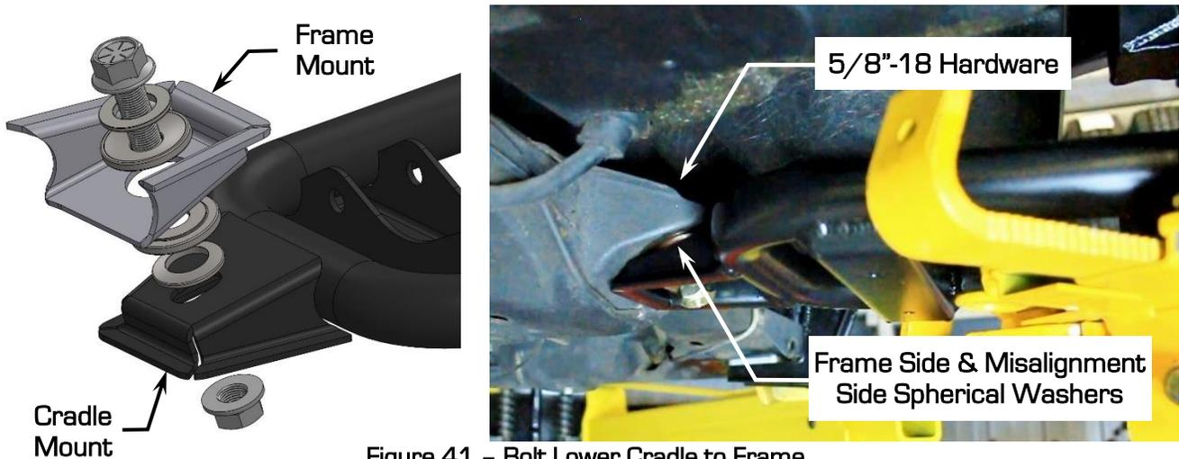
Figure 41 – Bolt Lower Cradle to Frame
