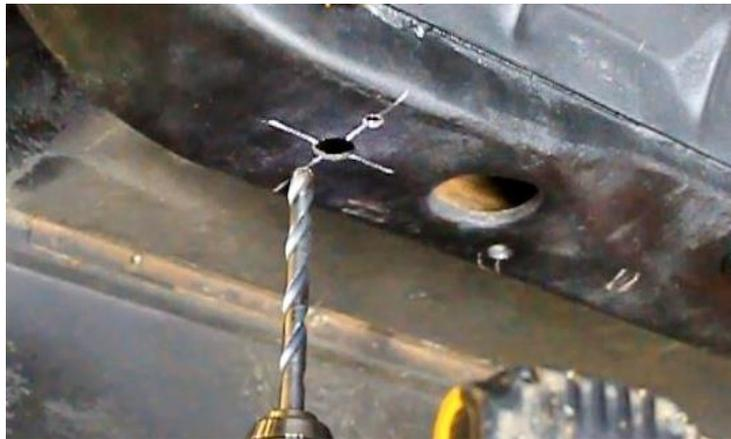
Figure 63 - Drill Sway Bar Nut Plate Location
