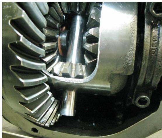
Figure 75 - Install Cross Shaft
