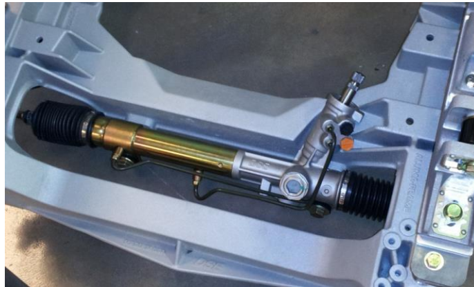
Figure 37 – Installed Rack & Pinion
