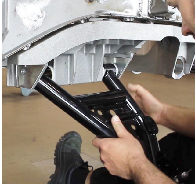
Figure 20 – Install Lower Control Arms
