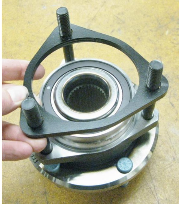
Figure 8 - Install Hub Shim
