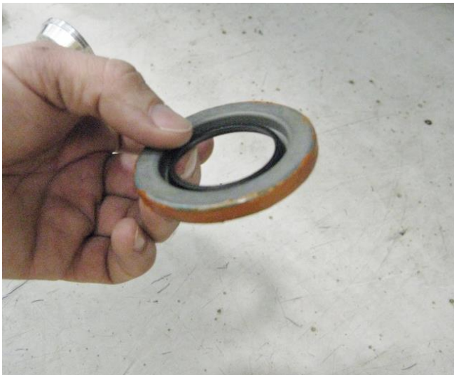
Figure 2 - Use RTV on the Axle Seals
