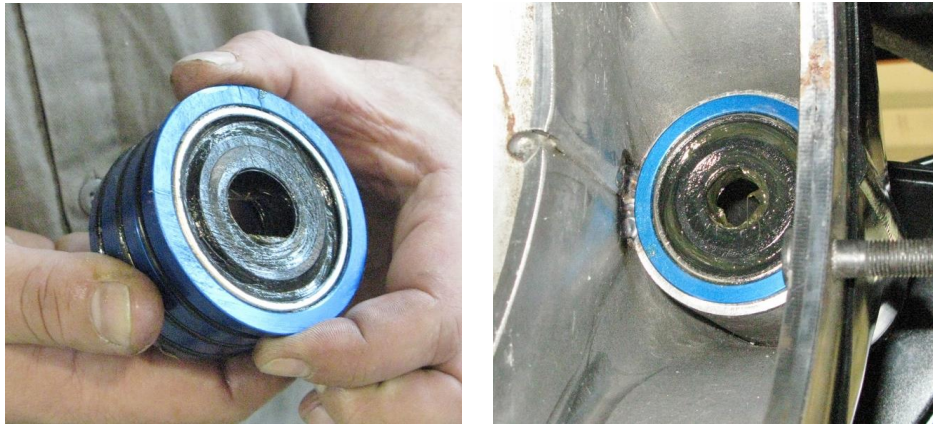
Figure 13 - Grease the Inner Axle Seals
