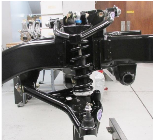
Figure 12 - Installed Coilover View (Passenger Side)
