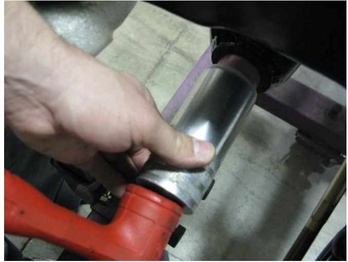
Figure 18 – Fully Installing the Bushings
