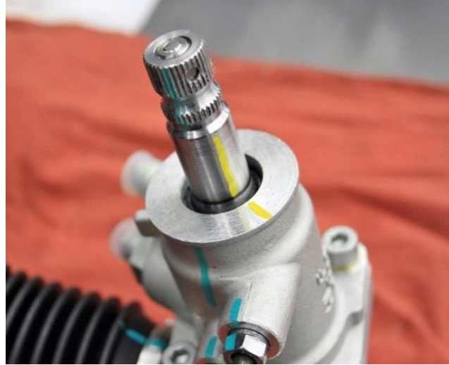
Figure 13 – Center the Rack & Pinion
