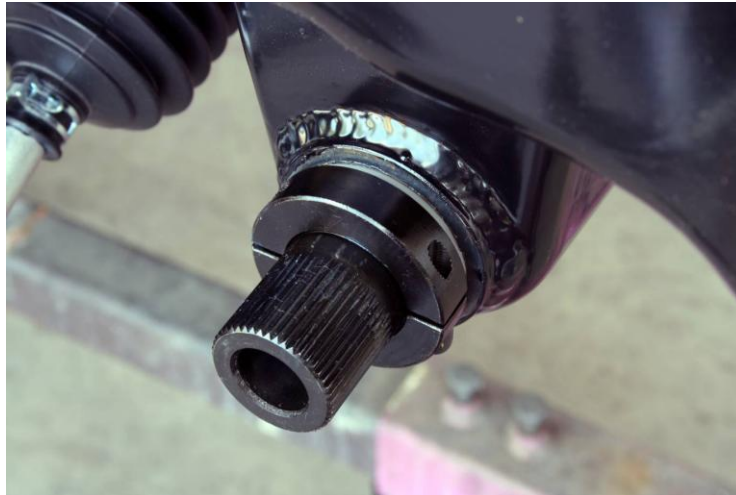
Figure 20 - Indexing the Clamp
