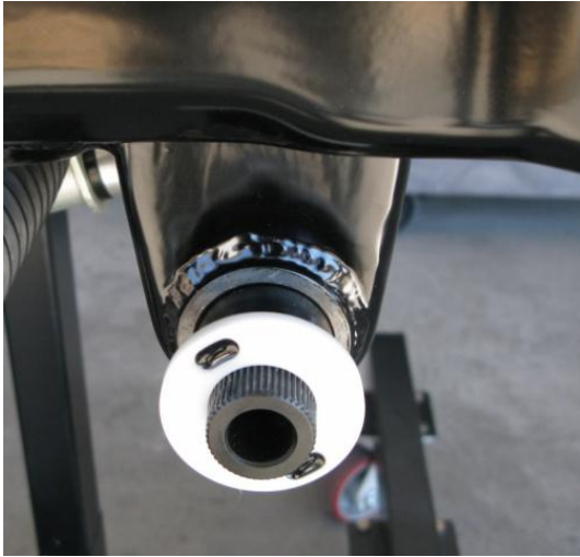
Figure 17 – Installing Bushing & Sway Bar
