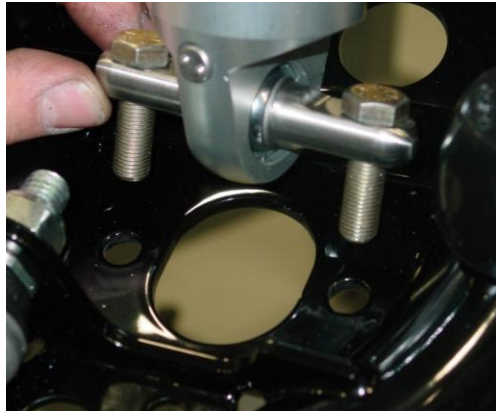
Figure 10 - Lower Shock Retaining Bolts
