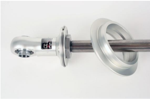
Figure 6 – Removing the Upper Spring Seat
