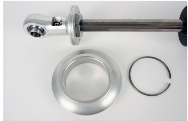
Figure 7 – Upper Spring Seat & Retaining Ring
