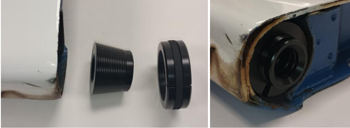
Insert Trunnion bushing into Tailgate
