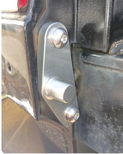
Install Trunnion Base, prepare for tailgate installation
