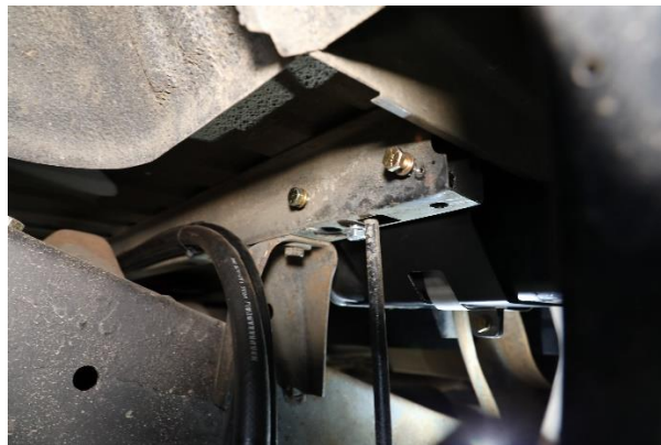
Figure 5 - Test Fit Bracket in Truck
