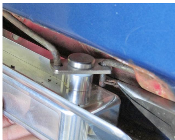
Install Tailgate Rods
