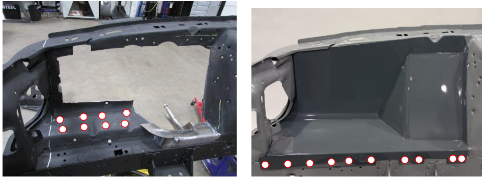
Figure 5 - Apron Panel Fitment and plug weld locations
